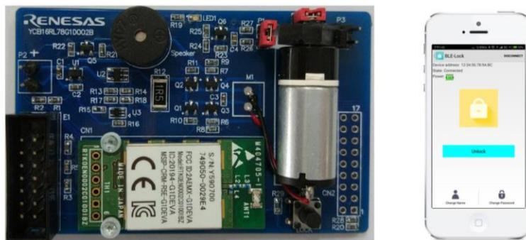
**Figure 6.** The smart lock system
