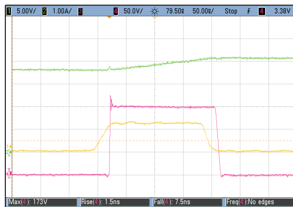
Figure 3. Waveforms for 150 VIN to 5 VOUT @ 4A (200 kHz) Buck Convertor. CH1: VPWM Input Voltage, CH2: Inductor Current, CH4: VOUT Switch Node Voltage
