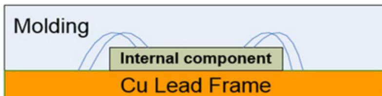
Figure 4. ISL8203M internal structure
