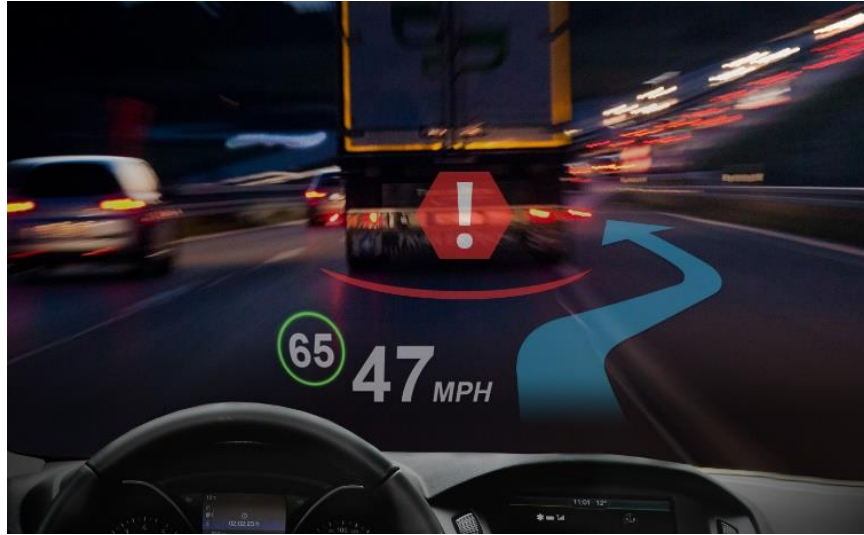
Figure 5. Laser head-up display presents full-HD video information in car driver's line of sight
