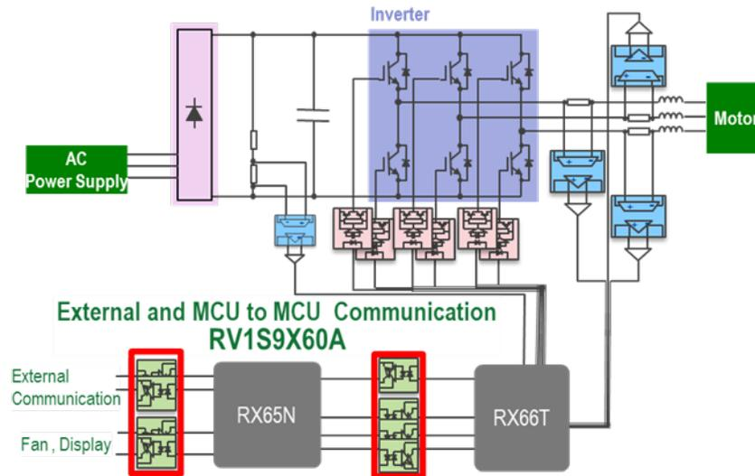
**Figure 1.** Inverter circuit of the general-purpose inverter.
