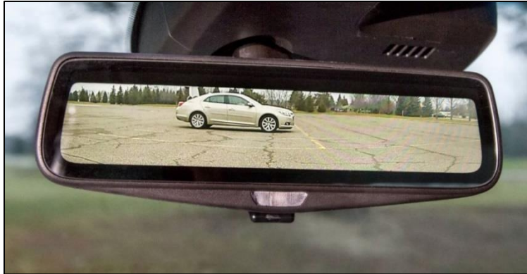
Figure 7. LCD rearview mirrors are beginning to replace reflective glass mirrors
