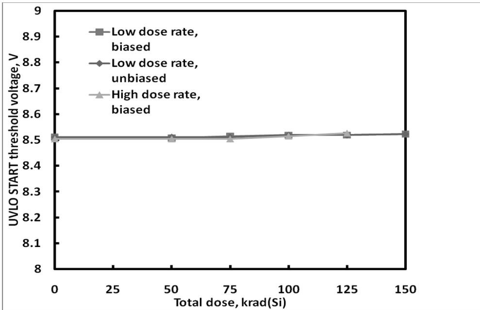
**Figure 3:** ISL78845ASRH undervoltage lockout START threshold voltage as a function of total dose irradiation at low and high dose rate. The low dose rate was 0.01rad(Si)/s and the high dose rate was 55rad(Si)/s. Sample size for each cell was 4. The post-irradiation SMD limits for this parameter are 8.0 – 9.0V.
