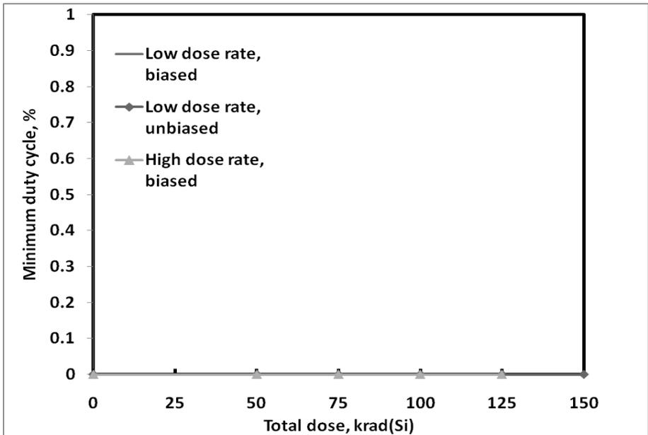
**Figure 16:** ISL78845ASRH minimum duty cycle as a function of total dose irradiation at low and high dose rate. The low dose rate was 0.01rad(Si)/s and the high dose rate was 55rad(Si)/s. Sample size for each cell was 4. The post-irradiation SMD limit for this parameter is 0% maximum. Note all plotted values were 0%.
