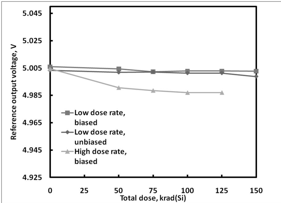
**Figure 7:** ISL78845ASRH master reference output voltage as a function of total dose irradiation at low and high dose rate. The low dose rate was 0.01rad(Si)/s and the high dose rate was 55rad(Si)/s. Sample size for each cell was 4. The post-irradiation SMD limits for this parameter are 4.925 – 5.050V.
