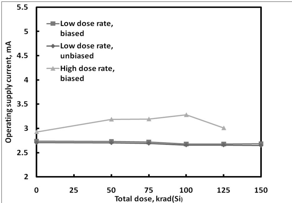
**Figure 6:** ISL78845ASRH operating supply current as a function of total dose irradiation at low and high dose rate. The low dose rate was 0.01rad(Si)/s and the high dose rate was 55rad(Si)/s. Sample size for each cell was 4. The post-irradiation SMD limit for this parameter is 5.5mA.
