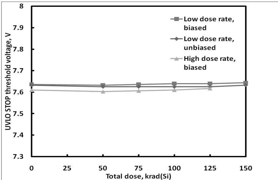
**Figure 4:** ISL78845ASRH undervoltage lockout STOP threshold voltage as a function of total dose irradiation at low and high dose rate. The low dose rate was 0.01rad(Si)/s and the high dose rate was 55rad(Si)/s. Sample size for each cell was 4. The post-irradiation SMD limits for this parameter are 7.3 – 8.0V.
