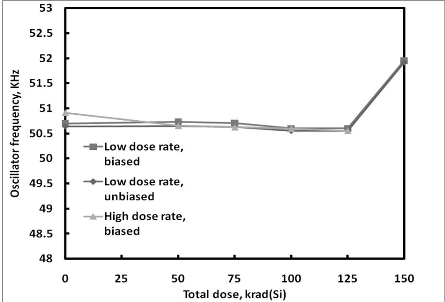
**Figure 14:** ISL78845ASRH oscillator frequency as a function of total dose irradiation at low and high dose rate. The low dose rate was 0.01rad(Si)/s and the high dose rate was 55rad(Si)/s. Sample size for each cell was 4. The post-irradiation SMD limits for this parameter are 48 – 53KHz.
