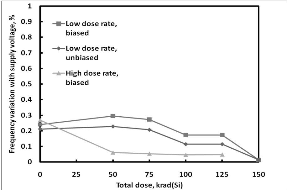
**Figure 15:** ISL78845ASRH oscillator frequency variation with  $V_{DD}$  as a function of total dose irradiation at low and high dose rate. The low dose rate was 0.01rad(Si)/s and the high dose rate was 55rad(Si)/s. Sample size for each cell was 4. The post-irradiation SMD limit for this parameter is 1% maximum.
