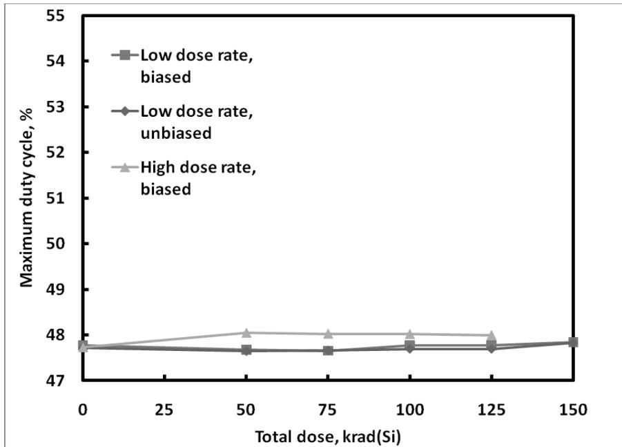
**Figure 17:** ISL78845ASRH maximum duty cycle as a function of total dose irradiation at low and high dose rate. The low dose rate was 0.01rad(Si)/s and the high dose rate was 55rad(Si)/s. Sample size for each cell was 4. The post-irradiation SMD limit for this parameter is 47% minimum.
