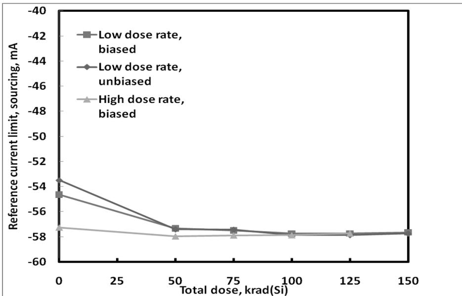
**Figure 8:** ISL78845ASRH reference current limit, sourcing, as a function of total dose irradiation at low and high dose rate. The low dose rate was 0.01rad(Si)/s and the high dose rate was 55rad(Si)/s. Sample size for each cell was 4. The post-irradiation SMD limit for this parameter is 20mA.
