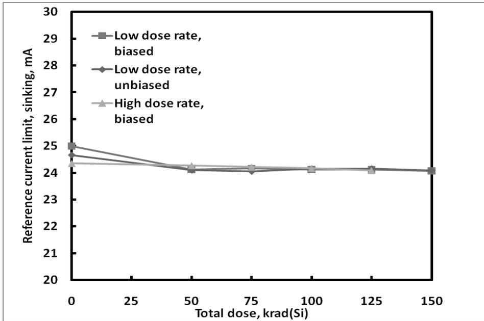
**Figure 9:** ISL78845ASRH reference current limit, sinking, as a function of total dose irradiation at low and high dose rate. The low dose rate was 0.01rad(Si)/s and the high dose rate was 55rad(Si)/s. Sample size for each cell was 4. The post-irradiation SMD limit for this parameter is 5mA minimum.
