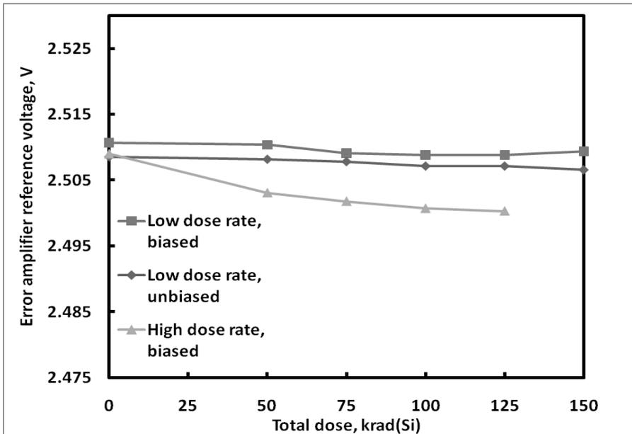
**Figure 12:** ISL78845ASRH error amplifier reference voltage as a function of total dose irradiation at low and high dose rate. The low dose rate was 0.01rad(Si)/s and the high dose rate was 55rad(Si)/s. Sample size for each cell was 4. The post-irradiation SMD limits for this parameter are 2.475 – 2.530V.
