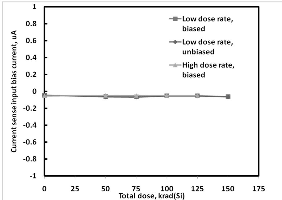
**Figure 10:** ISL78845ASRH current sense amplifier input bias current as a function of total dose irradiation at low and high dose rate. The low dose rate was 0.01rad(Si)/s and the high dose rate was 55rad(Si)/s. Sample size for each cell was 4. The post-irradiation SMD limits for this parameter are -1.0 – 1.0uA.
