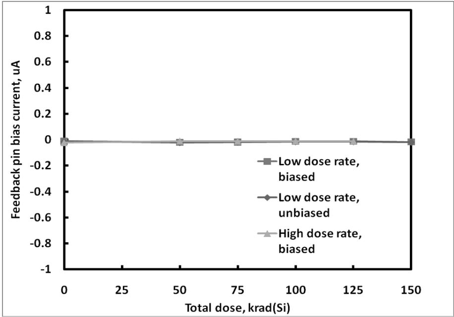
**Figure 13:** ISL78845ASRH error amplifier feedback pin bias current as a function of total dose irradiation at low and high dose rate. The low dose rate was 0.01rad(Si)/s and the high dose rate was 55rad(Si)/s. Sample size for each cell was 4. The post-irradiation SMD limits for this parameter are -1.0 – 1.0uA.
