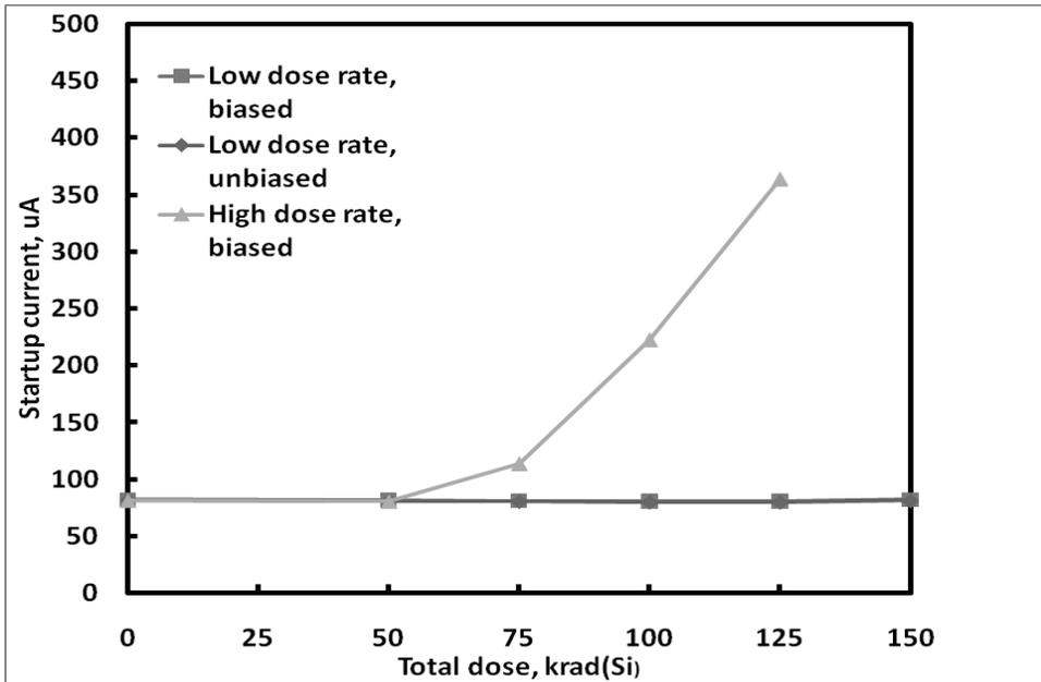
**Figure 5:** ISL78845ASRH startup current as a function of total dose irradiation at low and high dose rate. The low dose rate was 0.01rad(Si)/s and the high dose rate was 55rad(Si)/s. Sample size for each cell was 4. The SMD limit for this parameter is 125uA maximum pre-irradiation and 500uA post-irradiation.
