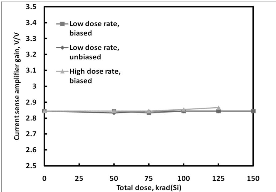
**Figure 11:** ISL78845ASRH current sense amplifier gain as a function of total dose irradiation at low and high dose rate. The low dose rate was 0.01rad(Si)/s and the high dose rate was 55rad(Si)/s. Sample size for each cell was 4. The post-irradiation SMD limits for this parameter are 2.5 – 3.5V/V.
