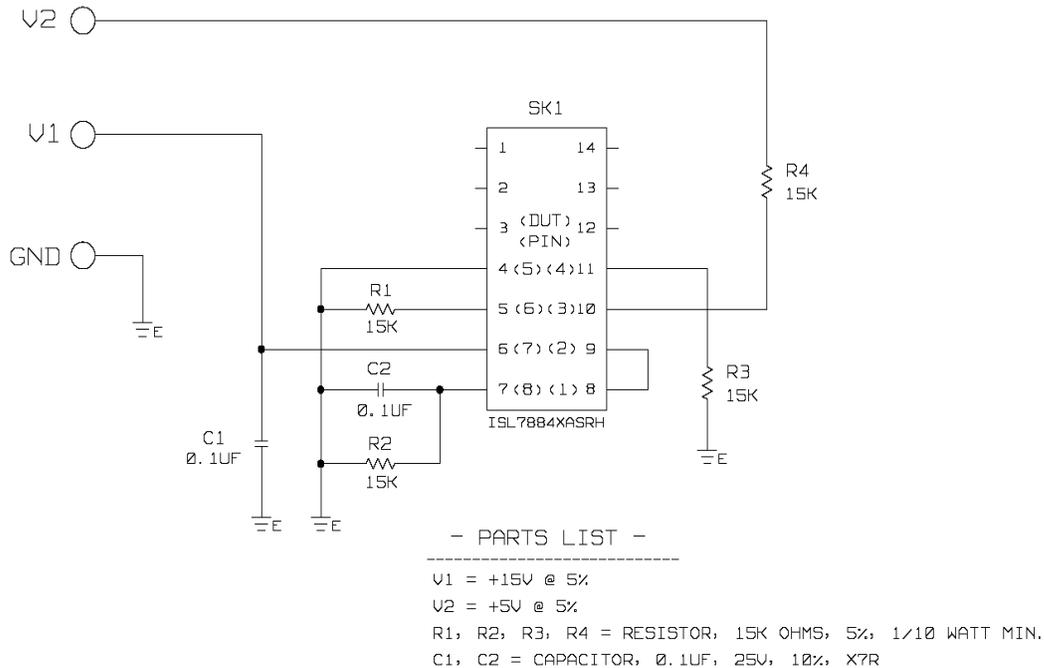
**Figure 2:** Irradiation bias configuration for the ISL78845ASRH per Standard Microcircuit Drawing (SMD) 5962-07249, as used for both low and high dose rate irradiation.
