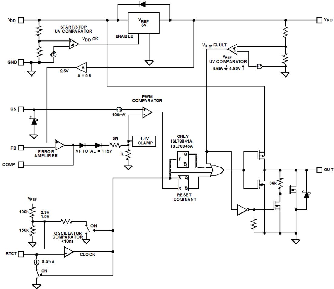
Figure 1: ISL78845ASRH block diagram.
