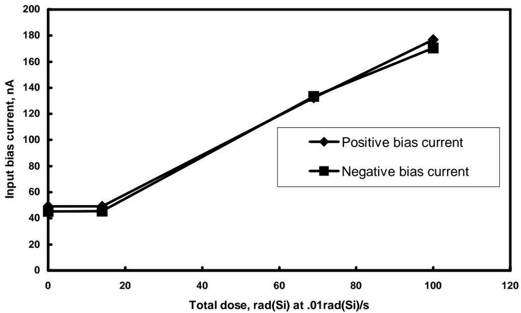
**Figure 4:** HS9-139RH average input bias current, positive and negative (inverting/noninverting) inputs, as a function of total dose. Sample size is 18 parts. The maximum post-radiation input bias current specification is 1uA.
