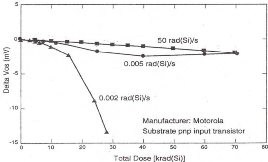
**Figure 1:** *Where is the bottom?* Degradation of the input bias current of the Motorola LM328 operational amplifier at three dose rates [1]. Note that the input offset voltage as a function of total dose shows excellent stability at the 50rad(Si)/s and .005rad(Si)/s dose rates, but degrades rapidly at the very low .002rad(Si)/s dose rate.
