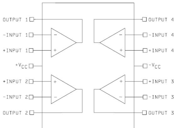
Fig. 1: HS-OP470AEH block diagram.
