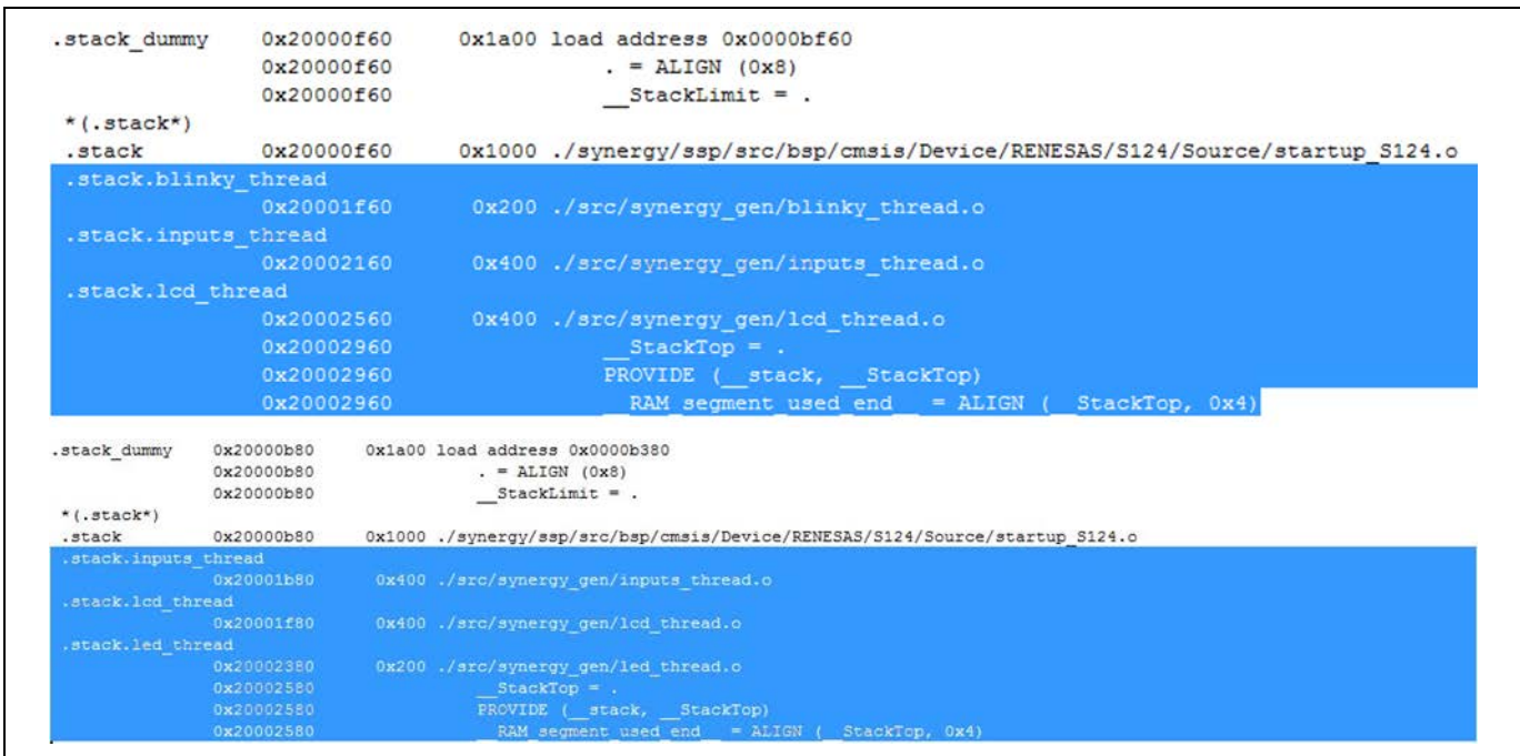
Figure 12. Locating thread stack addresses using the .map file
