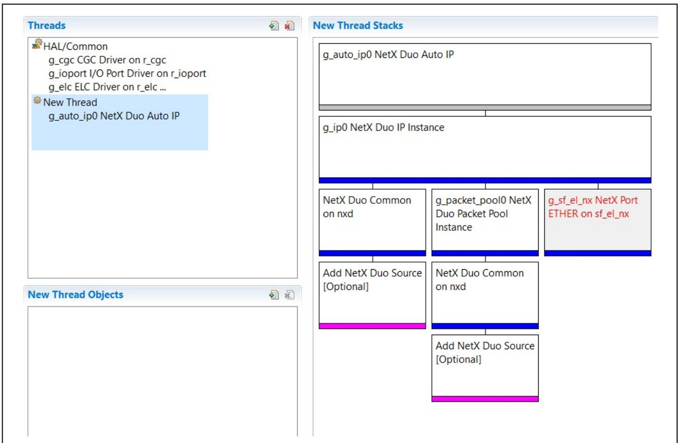
Figure 4. NetX Port Ether Application using NetX Duo Auto IP
