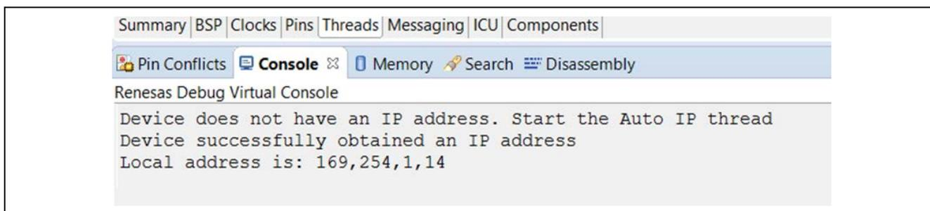
Figure 7. Example Output from NetX Port ETHER / Auto IP Application Project
