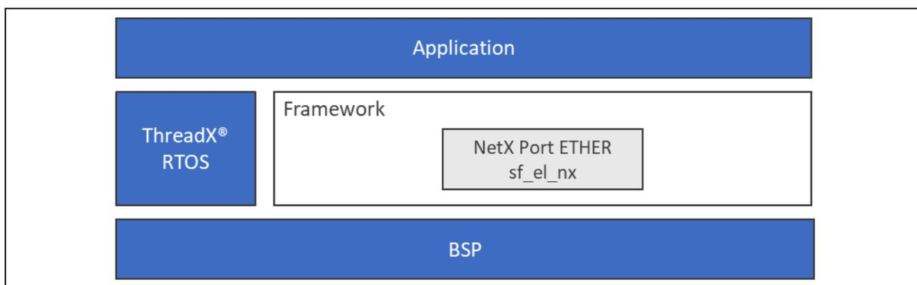
Figure 1. NetX Port Ether Module Block Diagram
