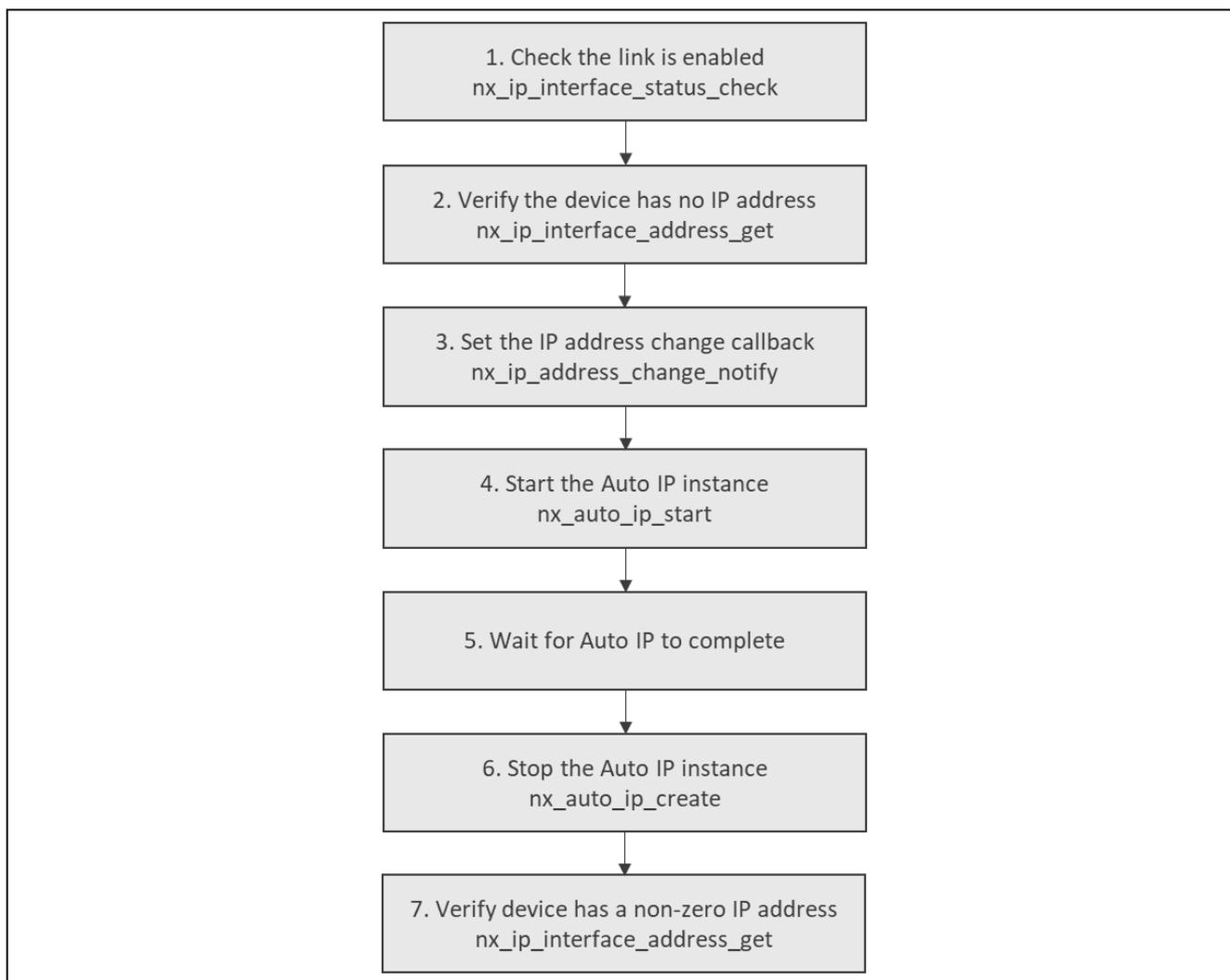
Figure 5. Flow Diagram of a Typical NetX Port Ether Module Application
