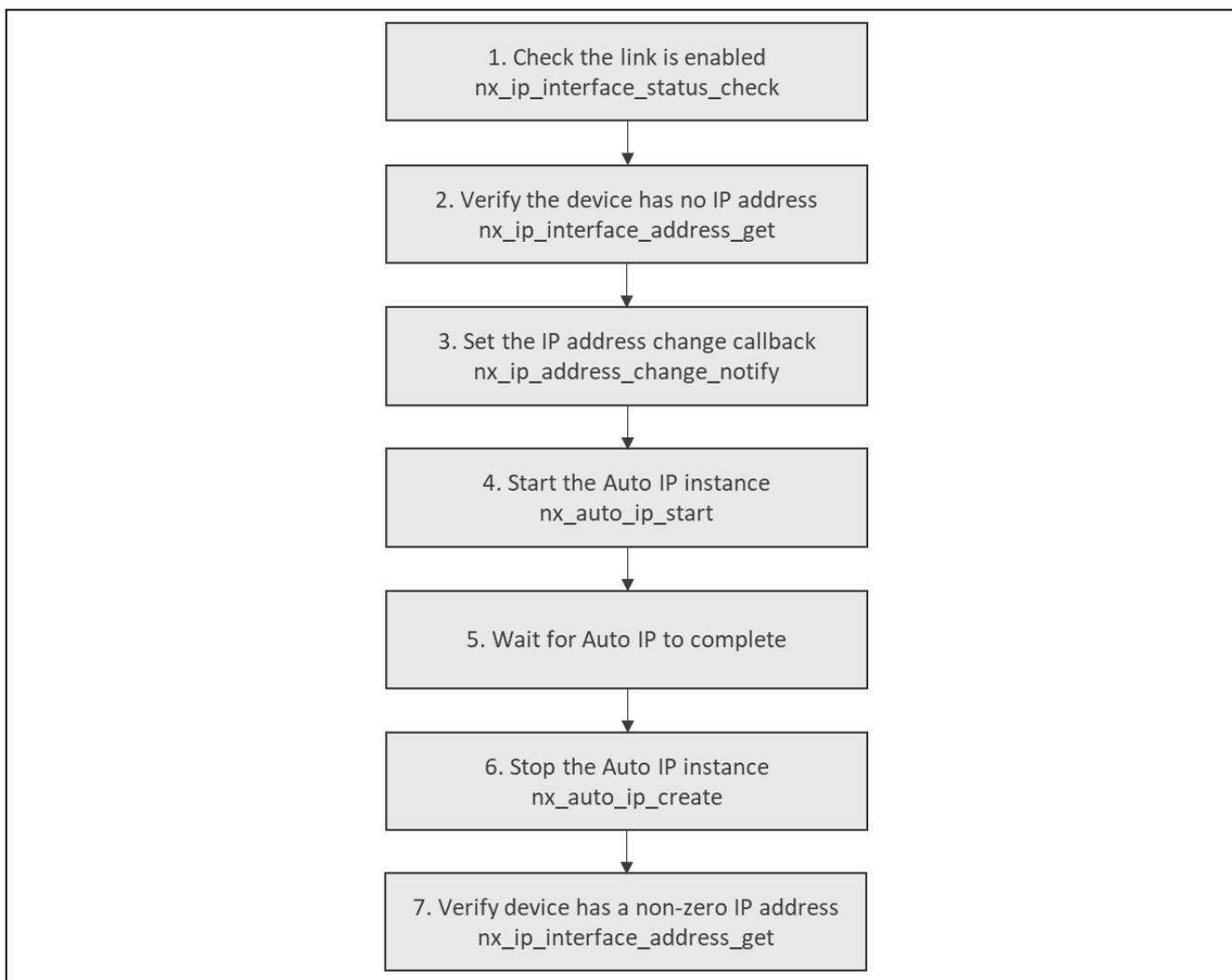
**Figure 6. NetX Port Ether Module Application Project Flow Diagram**
