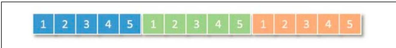
Figure 2. ADC Periodic Operation – Sample Order
