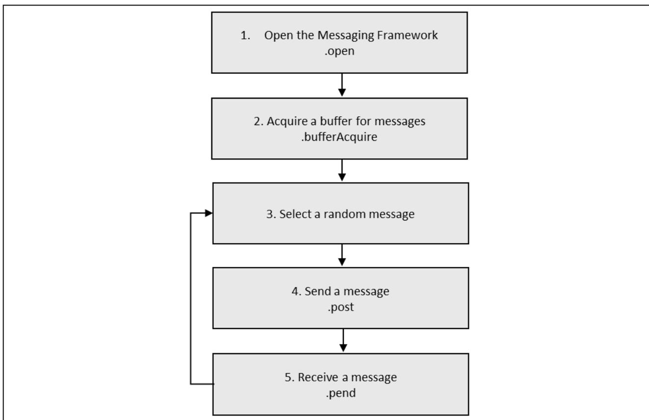
**Figure 13. Messaging Framework Module Application Project Flow Diagram**
