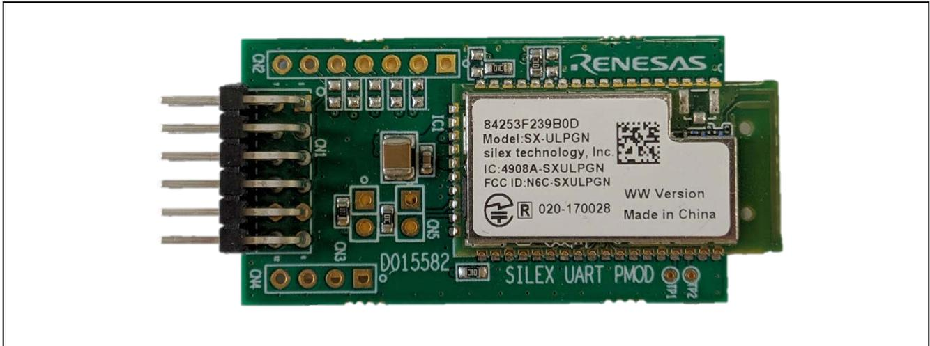
Figure 1. Wi-Fi Pmod™ Expansion Board
