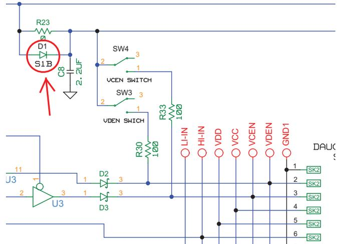
FIGURE 3. DIODE TO SUPPRESS LI-ON BATTERY RIPPLE
