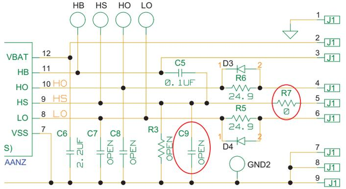
FIGURE 7. RC FILTER ON HS PIN (NOT REQUIRED)
