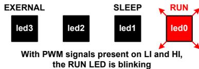
The DIP switch options are read only when the Start/Stop button is pressed to start the PWM signals. Changing the settings while the RUN LED is flashing will have no effect. To update the DIP switch setting, change the setting, stop the PWM signals, then start again.
