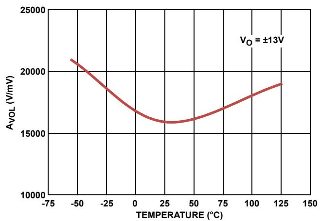
FIGURE 12.  $A_{VOL}$  vs TEMPERATURE
