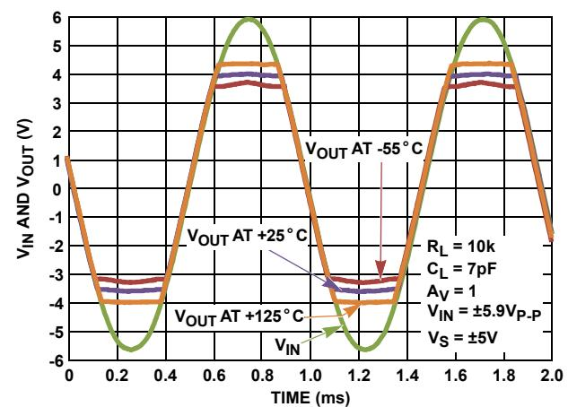
FIGURE 42. OUTPUT PHASE REVERSAL RESPONSE vs TEMPERATURE
