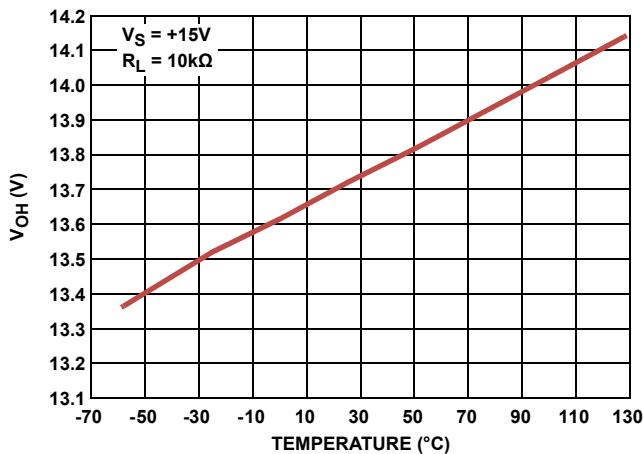
FIGURE 19.  $V_{OUT}$  vs TEMPERATURE
