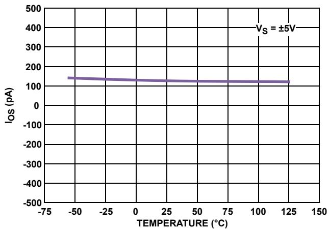
FIGURE 10.  $I_{OS}$  vs TEMPERATURE
