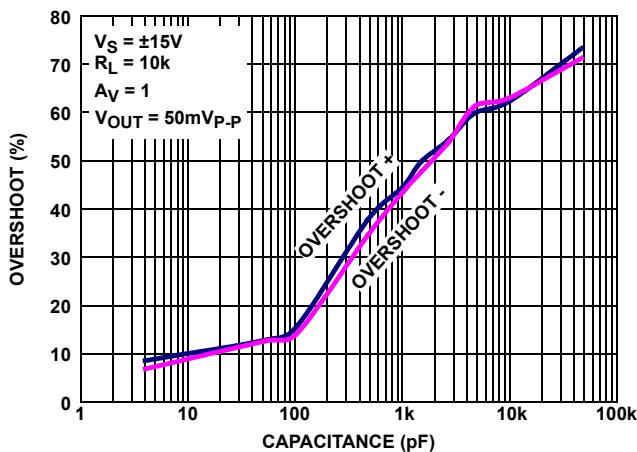
FIGURE 41. % OVERSHOOT vs LOAD CAPACITANCE,  $V_S = \pm 15V$
