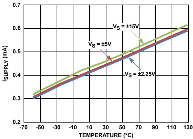
FIGURE 11. SUPPLY CURRENT PER AMPLIFIER vs TEMPERATURE
