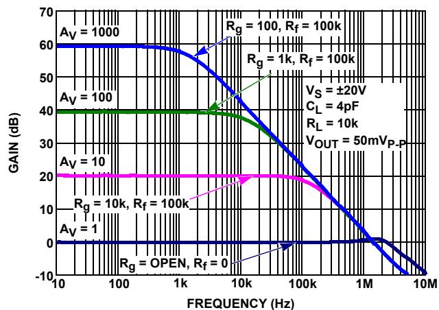
FIGURE 30. FREQUENCY RESPONSE vs CLOSED LOOP GAIN
