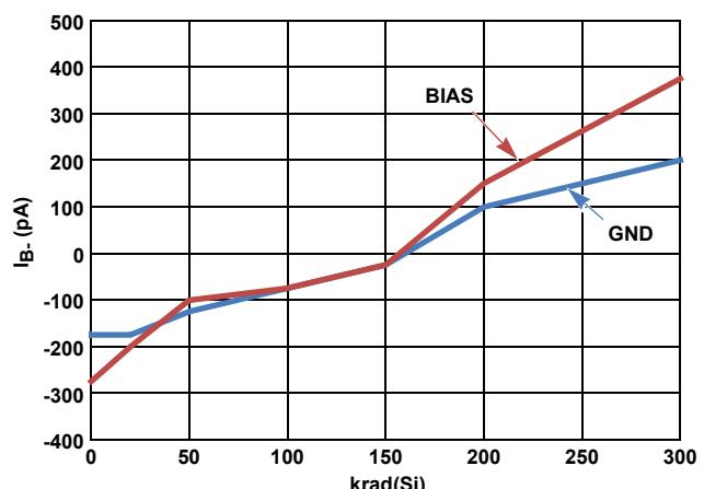
FIGURE 46. I<sub>B-</sub> vs HIGH DOSE RATE RADIATION
