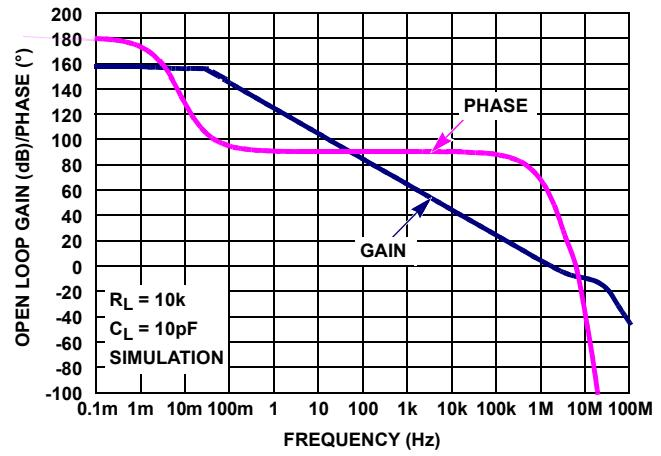
FIGURE 26. OPEN-LOOP GAIN, PHASE vs FREQUENCY,  $R_L = 10k\Omega$ ,  $C_L = 10\text{pF}$
