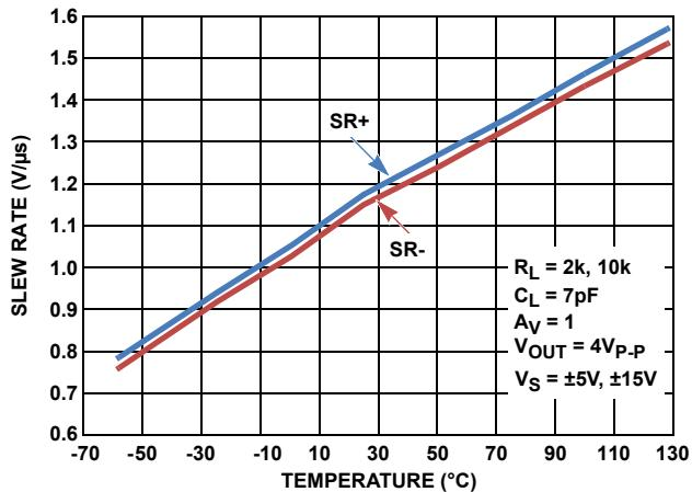
FIGURE 37. SLEW RATE vs TEMPERATURE  $V_S = \pm 5V, \pm 15V$
