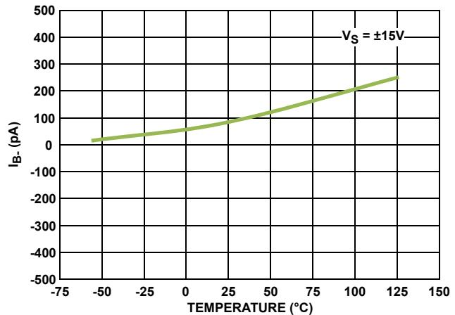
FIGURE 6.  $I_{B-}$  vs TEMPERATURE
