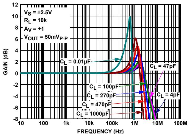
FIGURE 33. GAIN vs FREQUENCY vs  $C_L$
