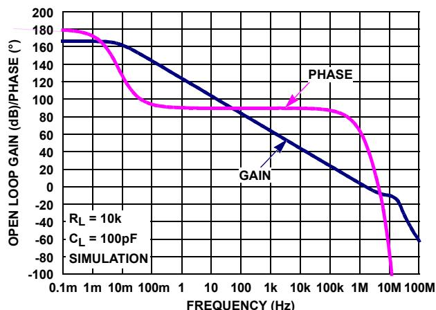
FIGURE 27. OPEN-LOOP GAIN, PHASE vs FREQUENCY,  $R_L = 10\text{k}\Omega$ ,  $C_L = 100\text{pF}$
