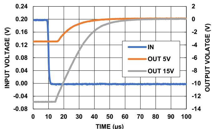
FIGURE 40. NEGATIVE OUTPUT OVERLOAD RESPONSE TIME,
