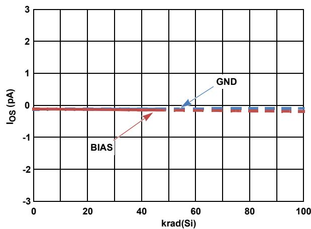
FIGURE 52.  $I_{OS}$  vs LOW DOSE RATE RADIATION
