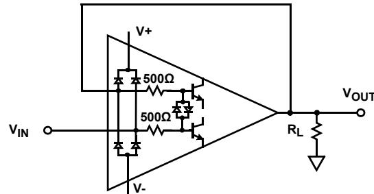
FIGURE 53. INPUT ESD DIODE CURRENT LIMITING - UNITY GAIN
