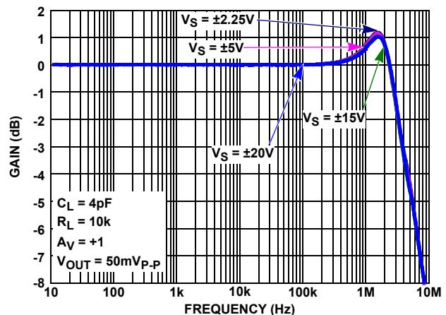
FIGURE 34. GAIN vs FREQUENCY vs SUPPLY VOLTAGE
