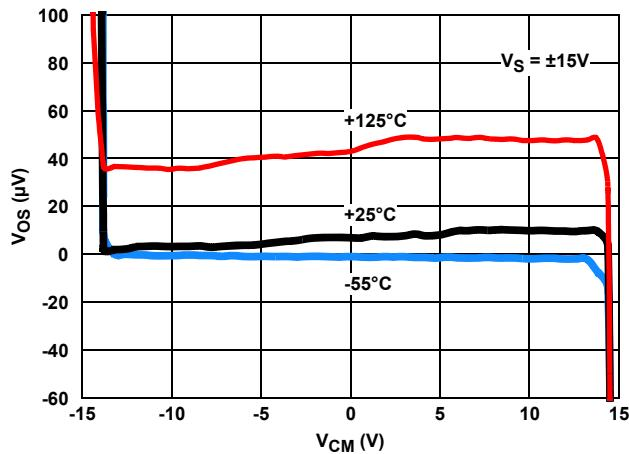
FIGURE 17. INPUT  $V_{OS}$  vs INPUT COMMON-MODE VOLTAGE,
