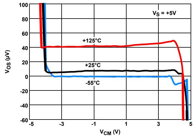
FIGURE 18. INPUT  $V_{OS}$  vs INPUT COMMON-MODE VOLTAGE,
