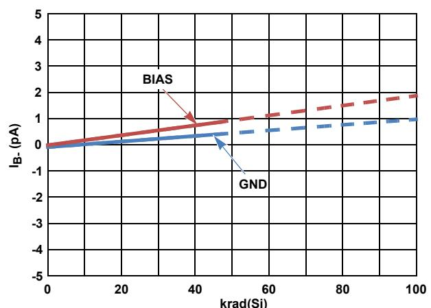
FIGURE 51.  $I_{B^-}$  vs LOW DOSE RATE RADIATION
