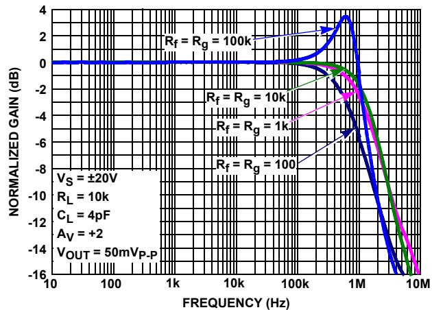
FIGURE 31. FREQUENCY RESPONSE vs FEEDBACK RESISTANCE  $R_f/R_g$
