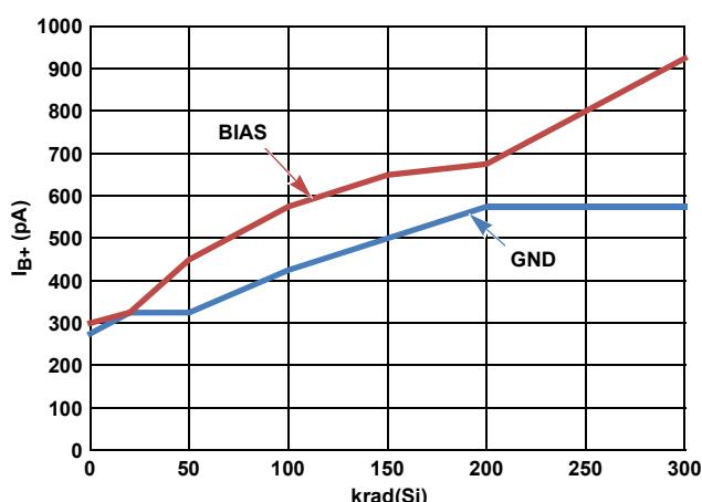
FIGURE 45. I<sub>B+</sub> vs HIGH DOSE RATE RADIATION
