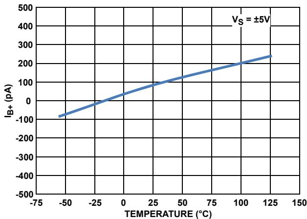
FIGURE 7.  $I_{B+}$  vs TEMPERATURE
