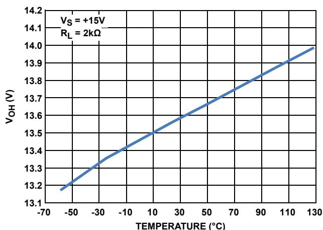
FIGURE 21.  $V_{OUT}$  vs TEMPERATURE
