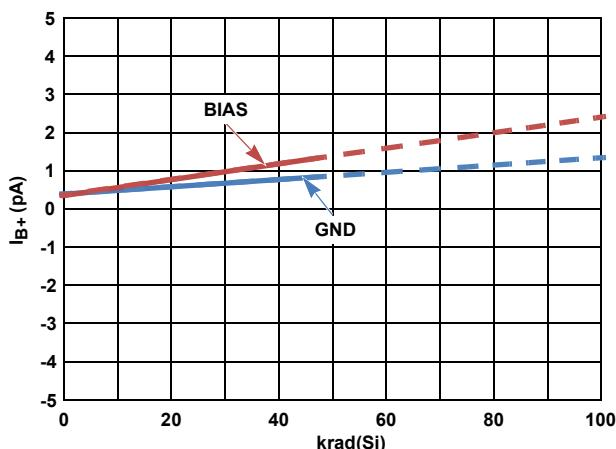
FIGURE 50.  $I_{B^+}$  vs LOW DOSE RATE RADIATION
