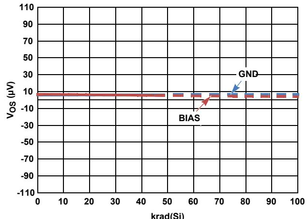
FIGURE 49.  $V_{OS}$  vs LOW DOSE RATE RADIATION
