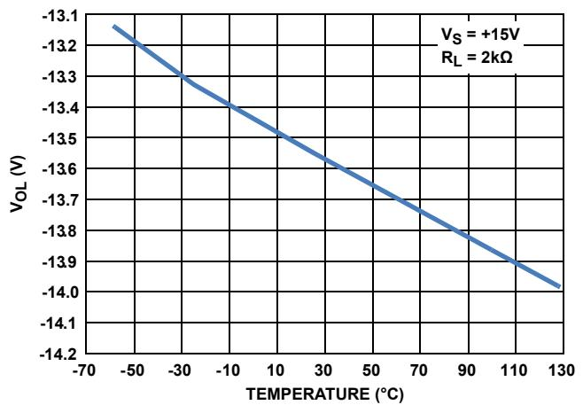
FIGURE 22.  $V_{OUT}$  vs TEMPERATURE
