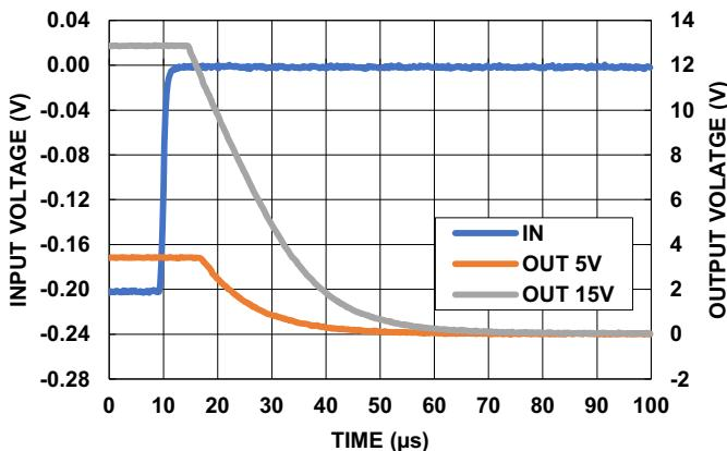
FIGURE 39. POSITIVE OUTPUT OVERLOAD RESPONSE TIME,
