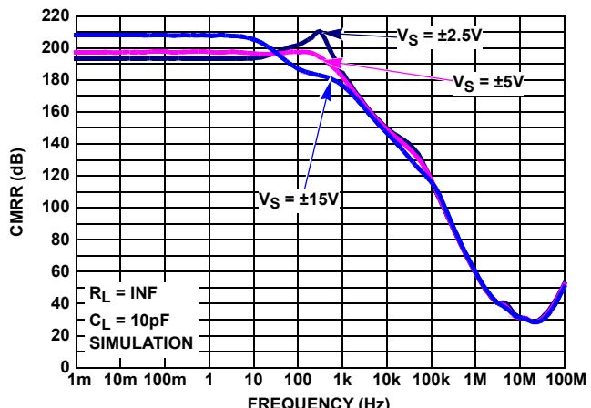
FIGURE 28. CMRR vs FREQUENCY,  $V_S = \pm 2.25, \pm 5V, \pm 15V$
