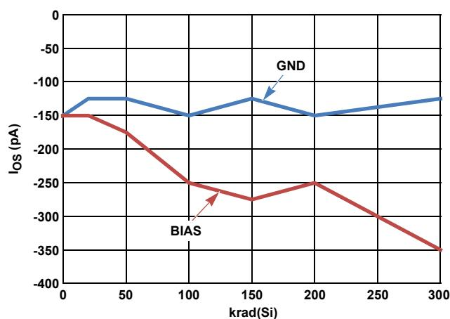
FIGURE 47. I<sub>OS</sub> vs HIGH DOSE RATE RADIATION
