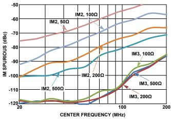
FIGURE 13. IM2 AND IM3 vs  $R_{LOAD}$
