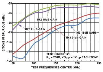
FIGURE 4. IM2 AND IM3 vs GAIN
