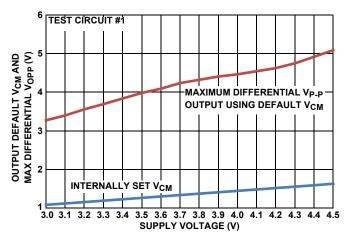
FIGURE 26. DEFAULT  $V_{\mbox{\footnotesize{CM}}}$  and max  $V_{\mbox{\footnotesize{OPP}}}$  vs supply voltage
