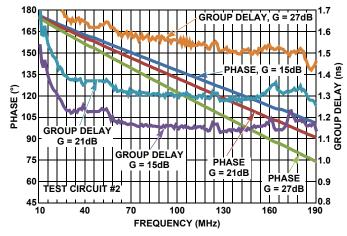
FIGURE 14. PHASE AND GROUP DELAY vs GAIN
