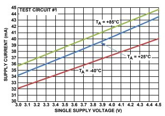
FIGURE 27. SUPPLY CURRENT vs SUPPLY VOLTAGE
