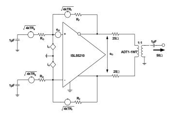
FIGURE 33. NOISE MODEL AND TEST CIRCUIT
