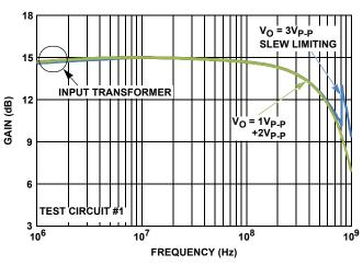
FIGURE 3. FREQUENCY RESPONSE vs OUTPUT SWING
