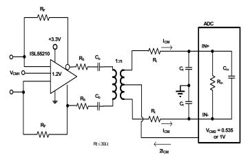
FIGURE 36. AC COUPLED WITH OUTPUT SIDE TRANSFORMER
