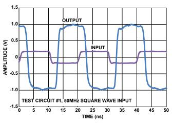
FIGURE 21. LARGE SIGNAL STEP RESPONSE
