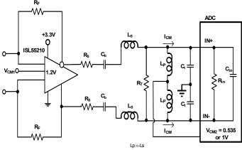
FIGURE 35. AC COUPLED, HIGHER FREQUENCY RLC FILTER DESIGN
