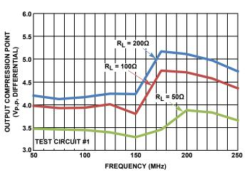
FIGURE 5. OUTPUT VP-P FOR -1dB GAIN COMPRESSION
