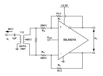
FIGURE 31. SINGLE TO DIFFERENTIAL WITH REDUCED FEEDBACK LOADING
