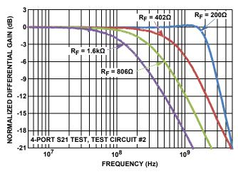
FIGURE 16. SMALL SIGNAL RESPONSE vs GAIN
