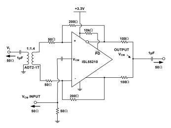
FIGURE 30. TEST CIRCUIT #3 COMMON MODE AC OUTPUT MEASUREMENTS
