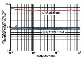
FIGURE 15. INPUT VOLTAGE AND CURRENT SPOT NOISE
