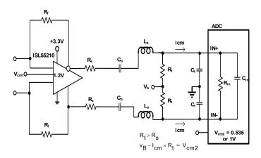
FIGURE 34. AC COUPLED, BROADBAND RLC INTERSTAGE FILTER DE SIGN
