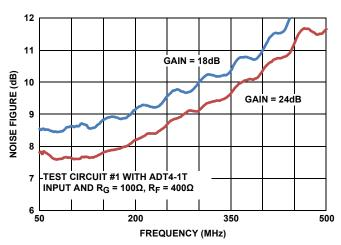
FIGURE 7. NOISE FIGURE AT HIGHER GAINS
