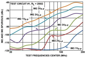
FIGURE 9. IM2 AND IM3 vs OUTPUT SWING
