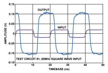
FIGURE 20. SMALL SIGNAL STEP RESPONSE
