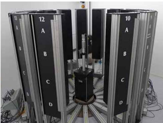
**Fig. 2:** View of the 'pop-up'  $^{60}\text{Co}$  source (center) and surrounding test racks. The board holders are arranged in an approximate sphere surrounding the source. All DUT boards are enclosed in PbAl spectrum hardening boxes to filter out secondary radiation. The total DUT board capacity is 64.
