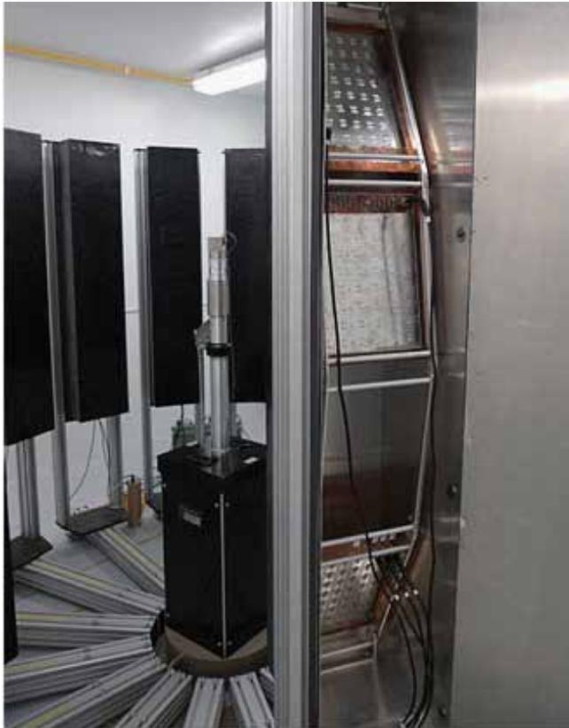
**Fig. 1:** Image showing a single vertical test board holder and PbAl spectrum hardening filter box with the access door open. The holder is on rails and can be moved towards the centrally located source as the source loses activity. The curvature of the DUT rack can be clearly seen.
