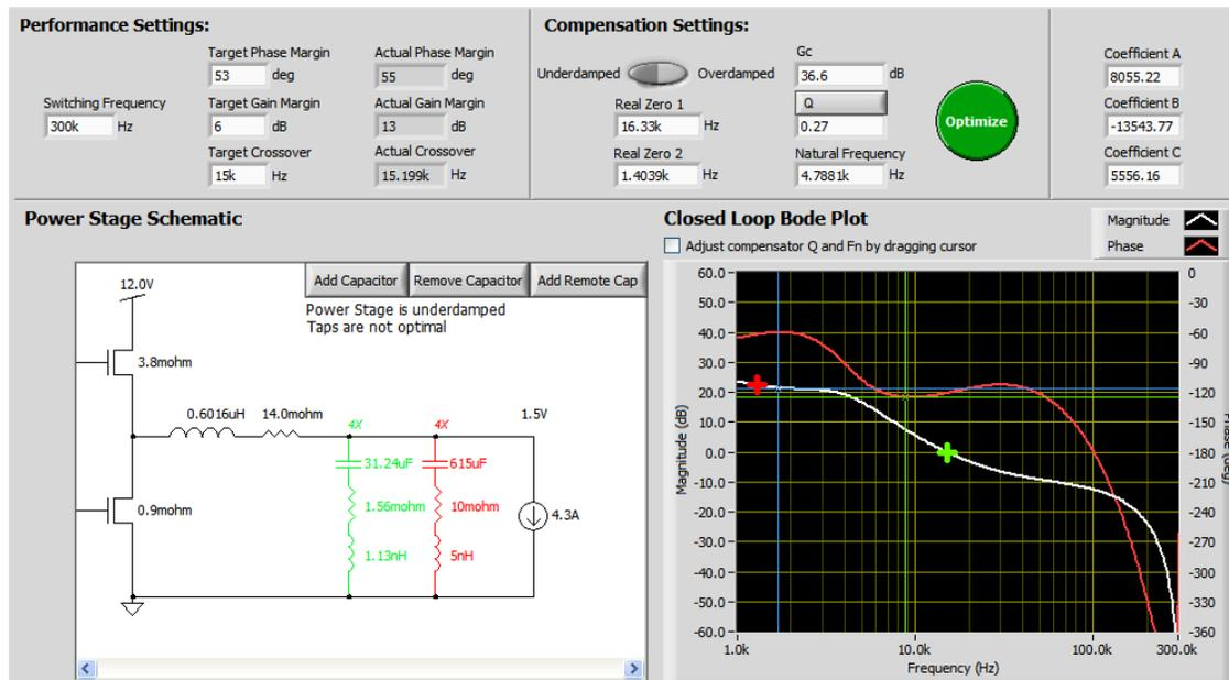
Figure 10. CompZL Manual Results, with Mid-Band Gain Boost
