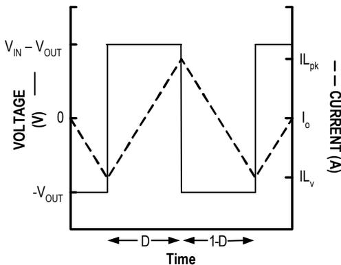
**Figure 2. Inductor Waveforms**
