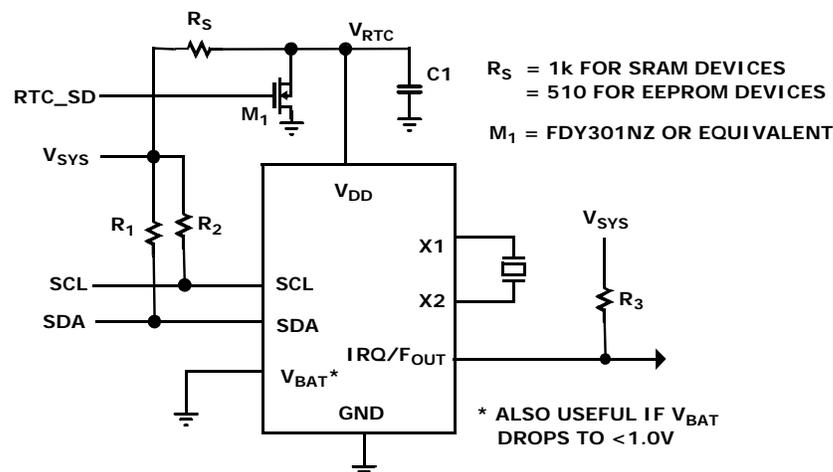
FIGURE 2. POWERING A DEVICE WITH NO BATTERY BACKUP
