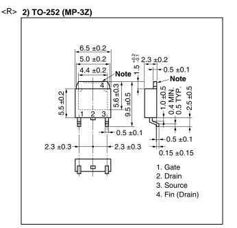
**Note** The depth of notch at the top of the fin is from 0 to 0.2 mm.
