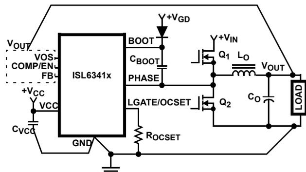
FIGURE 12. PRINTED CIRCUIT BOARD SMALL SIGNAL LAYOUT GUIDELINES
