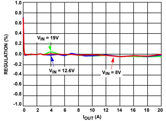
FIGURE 14. LOAD REGULATION AT  $V_{OUT} = 1.1V$
