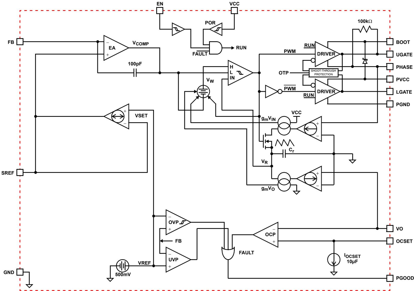
FIGURE 1. SIMPLIFIED FUNCTIONAL BLOCK DIAGRAM OF ISL62870
