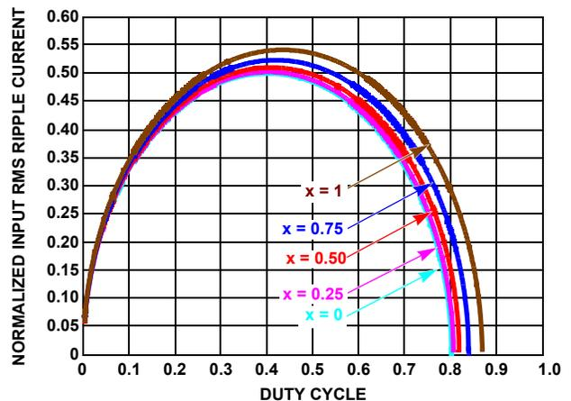
FIGURE 9. NORMALIZED RMS INPUT CURRENT FOR  $x = 0.8$
