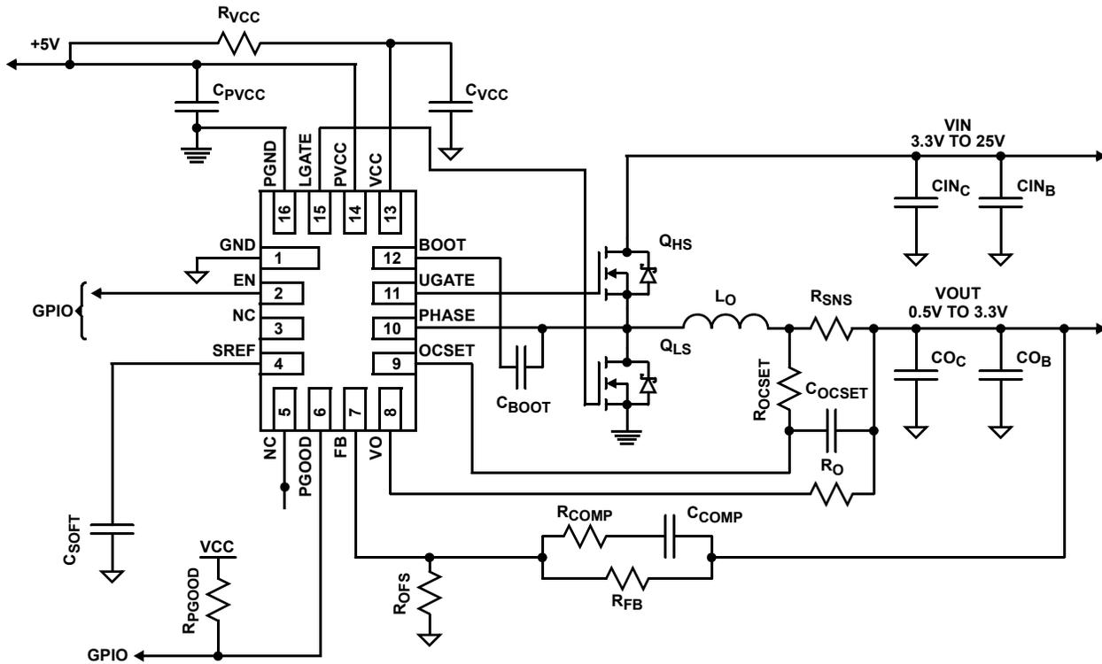
FIGURE 3. ISL62870 APPLICATION SCHEMATIC WITH RESISTOR CURRENT SENSE
