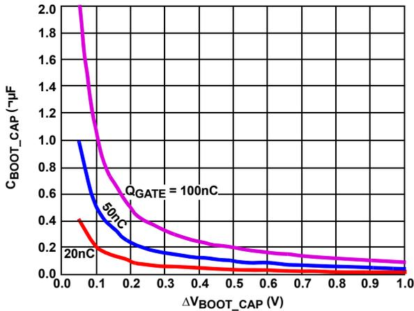
FIGURE 10. BOOTSTRAP CAPACITANCE vs BOOT RIPPLE VOLTAGE
