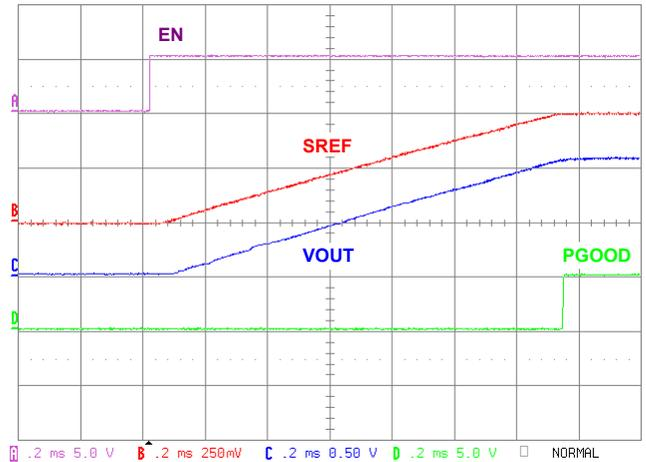
FIGURE 16. START-UP,  $V_{IN} = 12.6V$ ,  $V_{OUT} = 1.05V$ , LOAD = 10A
