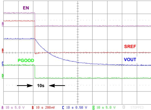
**FIGURE 19. SHUT-DOWN,  $V_{IN} = 12.6V$ ,  $V_{OUT} = 1.05V$ , LOAD = OPEN-CIRCUIT**
