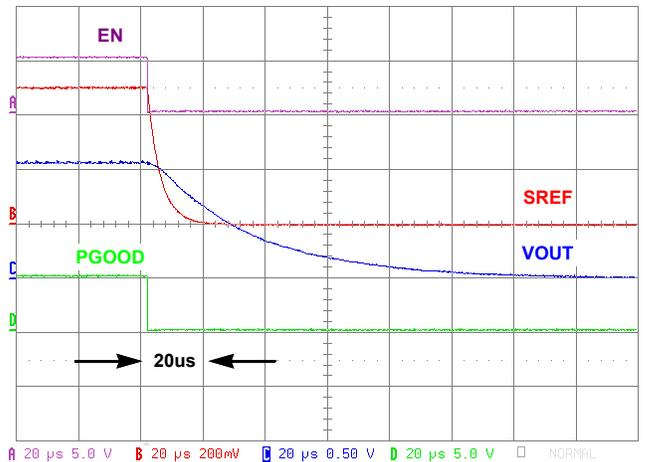
FIGURE 18. SHUT-DOWN,  $V_{IN} = 12.6V$ ,  $V_{OUT} = 1.05V$ , LOAD = 50mΩ
