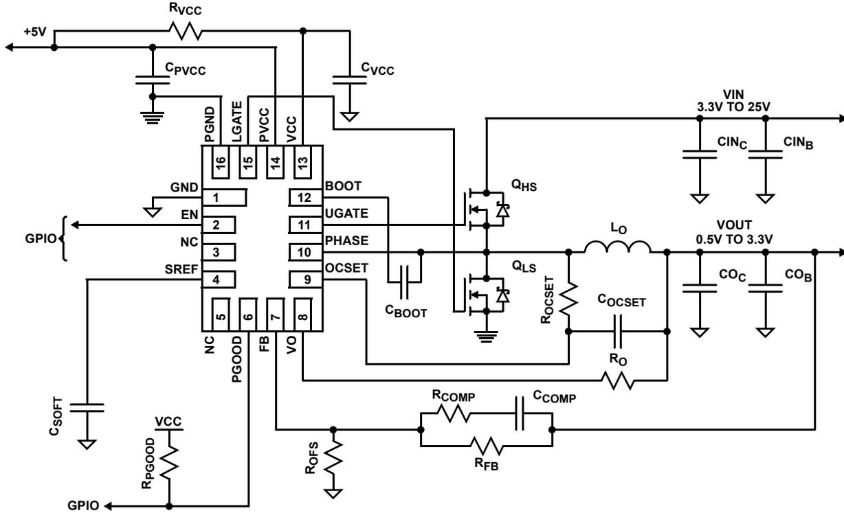
FIGURE 2. ISL62870 APPLICATION SCHEMATIC WITH DCR CURRENT SENSE
