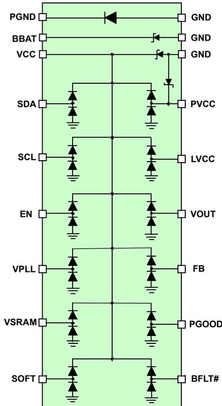
**FIGURE 26. INTERNAL ESD STRUCTURES**
