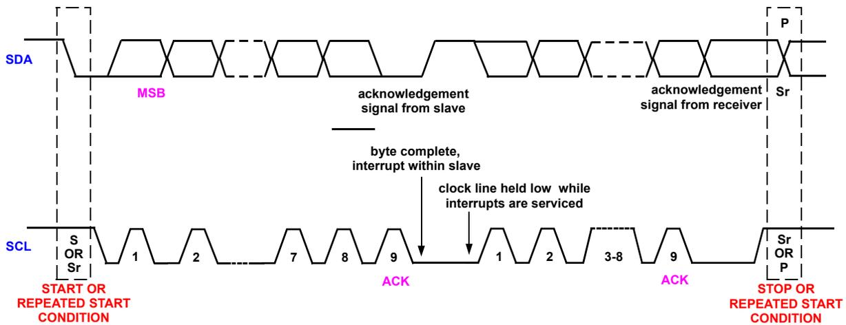
FIGURE 17. I<sup>2</sup>C DATA AND CLOCK
