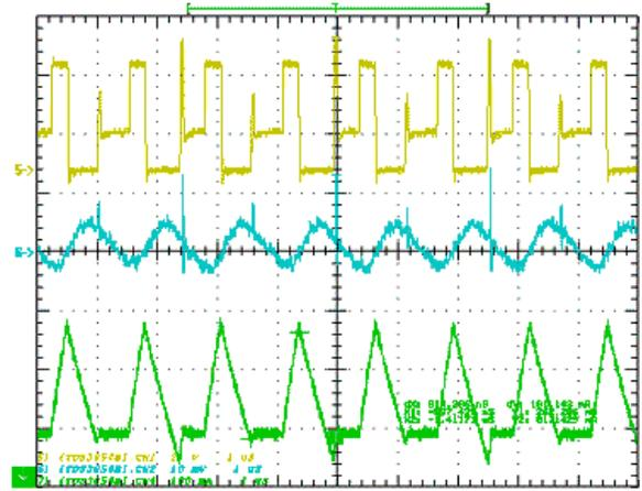
Top: phase node output voltage ripple, 10mV/DIV
