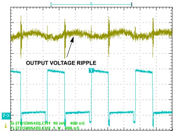
Ripple in CCM Vin = 2.85V, Vo = 0.850V, Fripple = 1MHz, I<sub>o</sub> = 500mA, Ripple = 4.2mV, 400ns/DIV
