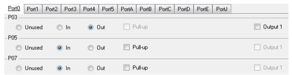
Figure 1 Example of Display when PORT0 is Set in R5F52315AxFP (100-pin)
