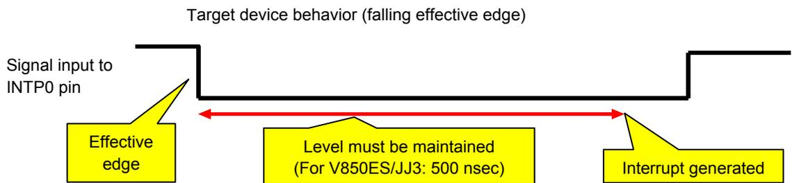
In the case of the simulator, however, this noise reduction circuit is not simulated. For this reason, an interrupt will be generated any time a valid edge is generated. (No need to maintain signal level).
