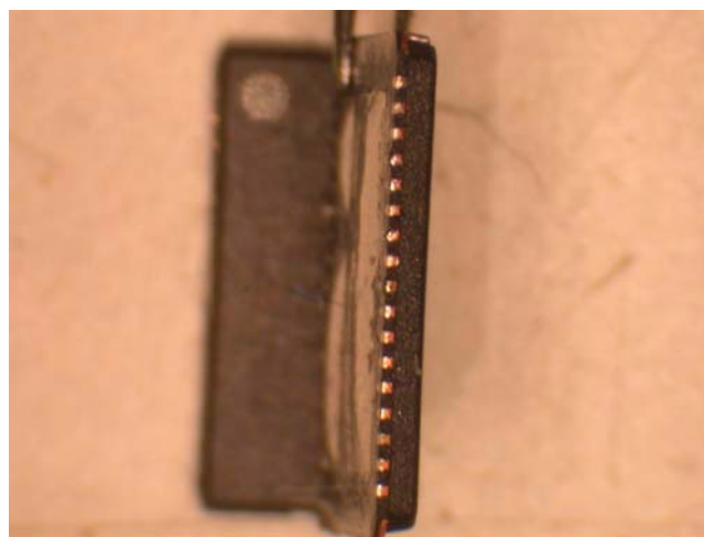
FIGURE 17. FINISHED TINNED THERMAL LAND ON QFN
