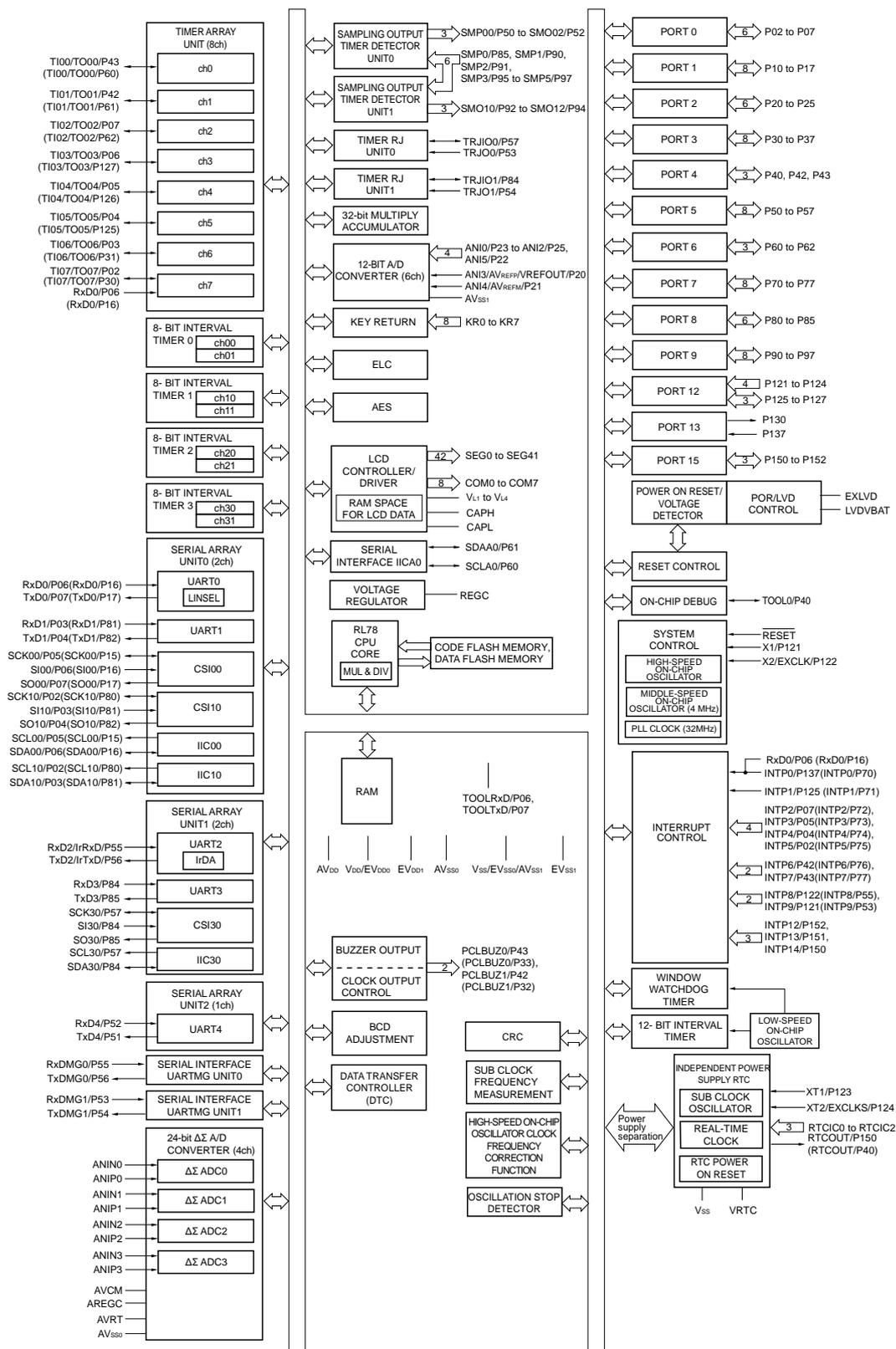
**Remark** Functions in parentheses in the above figure can be assigned via settings in the peripheral I/O redirection register (PIOR0). See **Figure 4-7 Format of Peripheral I/O Redirection Register (PIOR0)** in the RL78/I1C (512 KB) User's Manual.
