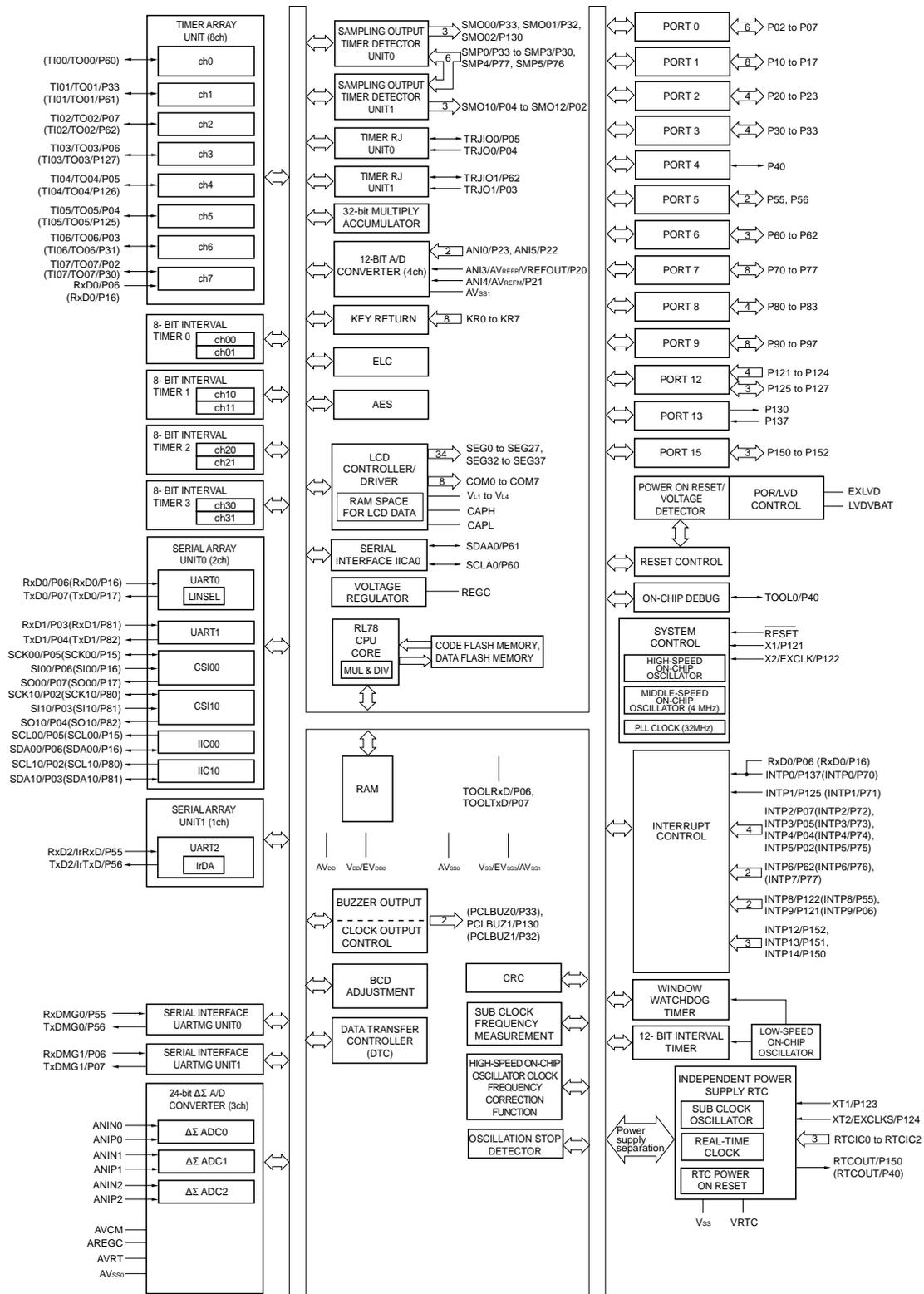
**Remark** Functions in parentheses in the above figure can be assigned via settings in the peripheral I/O redirection register (PIOR0). See **Figure 4-7 Format of Peripheral I/O Redirection Register (PIOR0)** in the RL78/I1C (512 KB) User's Manual.
