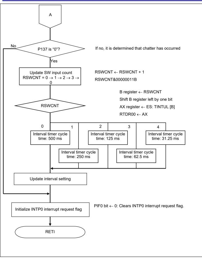
Figure 5.12 INTP0 Interrupt Processing (2/2)
