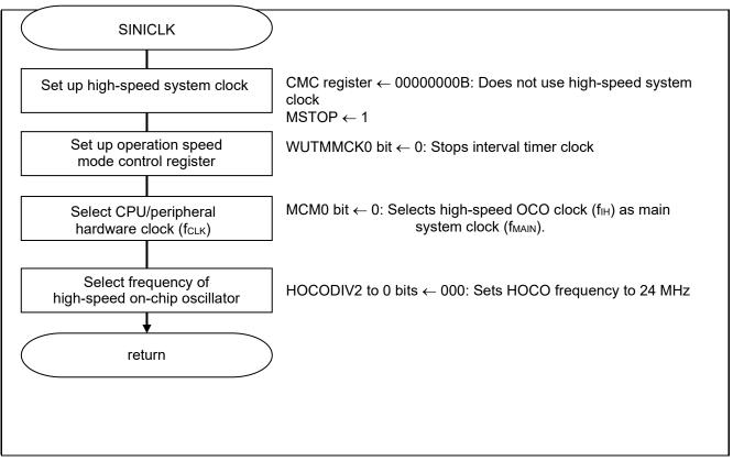
Figure 5.4 Clock Generation Circuit Setup
