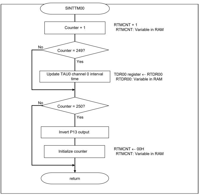
Figure 5.10 Flowchart for LED Turn-on/off Processing
