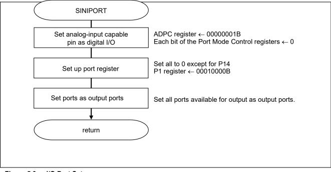
Figure 5.3 I/O Port Setup
