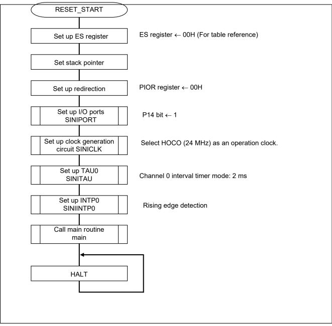
Figure 5.2 CPU Initialization Function
