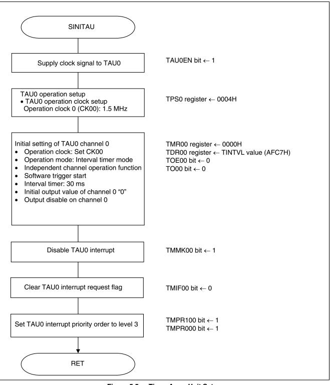
Figure 5.5 Timer Array Unit Setup
