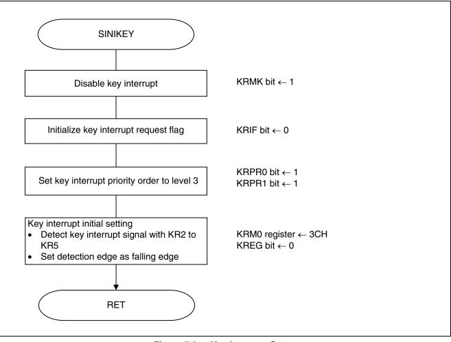
Figure 5.6 Key Interrupt Setup
