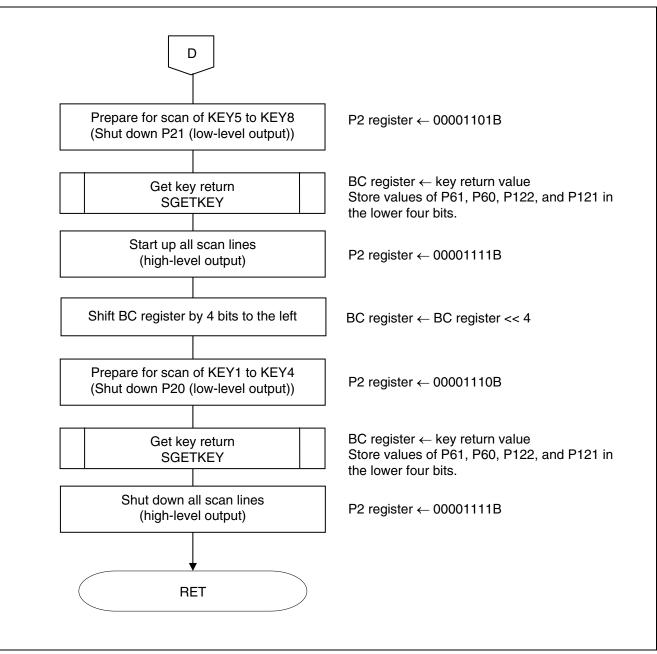
Figure 5.12 Detecting Input Key (2/2)
