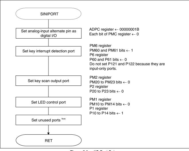
Figure 5.3 I/O Port Setup
