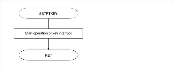
Figure 5.10 Enabling Key Interrupt
