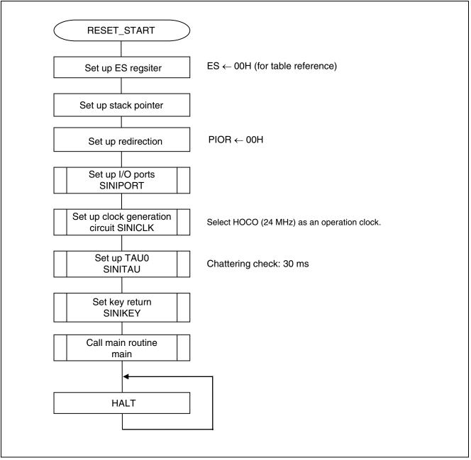
Figure 5.2 CPU Initialization Function
