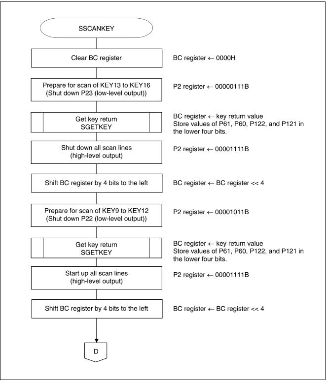
Figure 5.11 Detecting Input Key (1/2)
