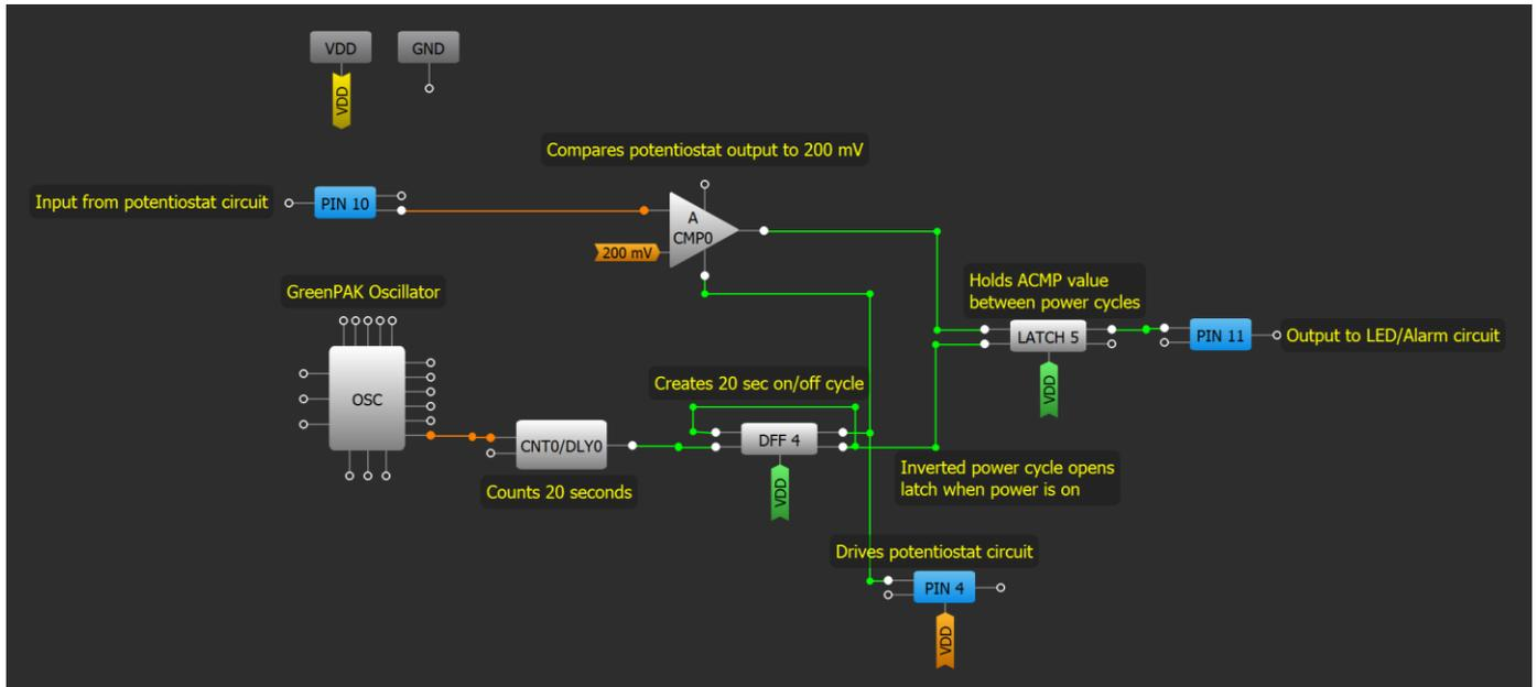
Figure 14. The internal connections of the GreenPAK4 blocks
