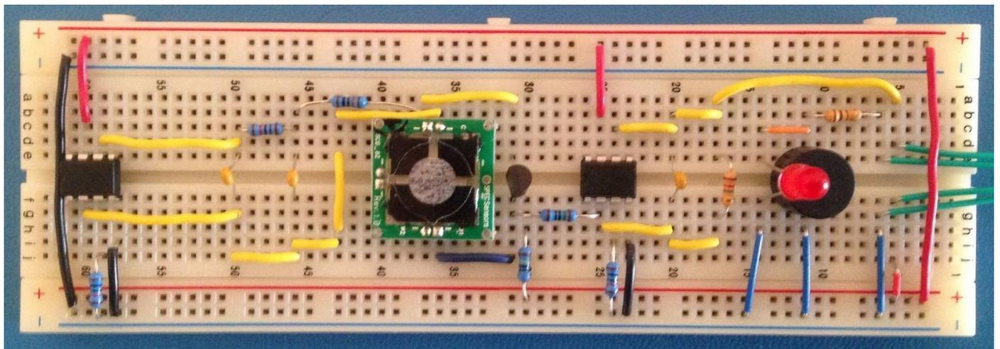
**Figure 3. The potentiostat and LED/Alarm circuit prototyped on a breadboard. The protruding green wires connect to the GreenPAK Universal Development Board. For a full list of the external components used, see Appendix**
