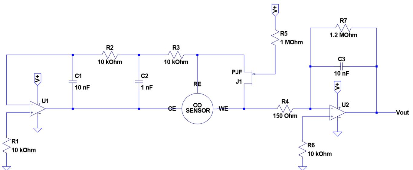
**Figure 1. The potentiostat schematic for the SPEC CO sensor 100-102. CE, RE, and WE stand for Counter Electrode, Reference Electrode, and Working Electrode, respectively**
