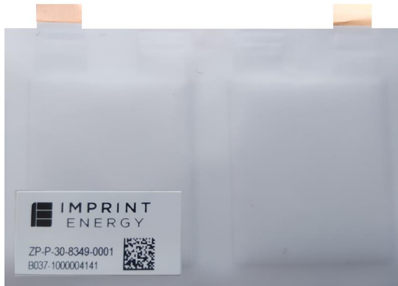
Figure 6: The actual 15mAh ZincPoly flex, ultra-thin battery
