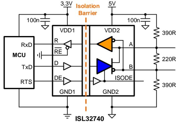
Figure 2. Modern PROFIBUS DP node using ISL32740
