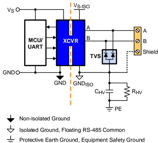
**Figure 3. Isolated PROFIBUS DP node with transient protection**
