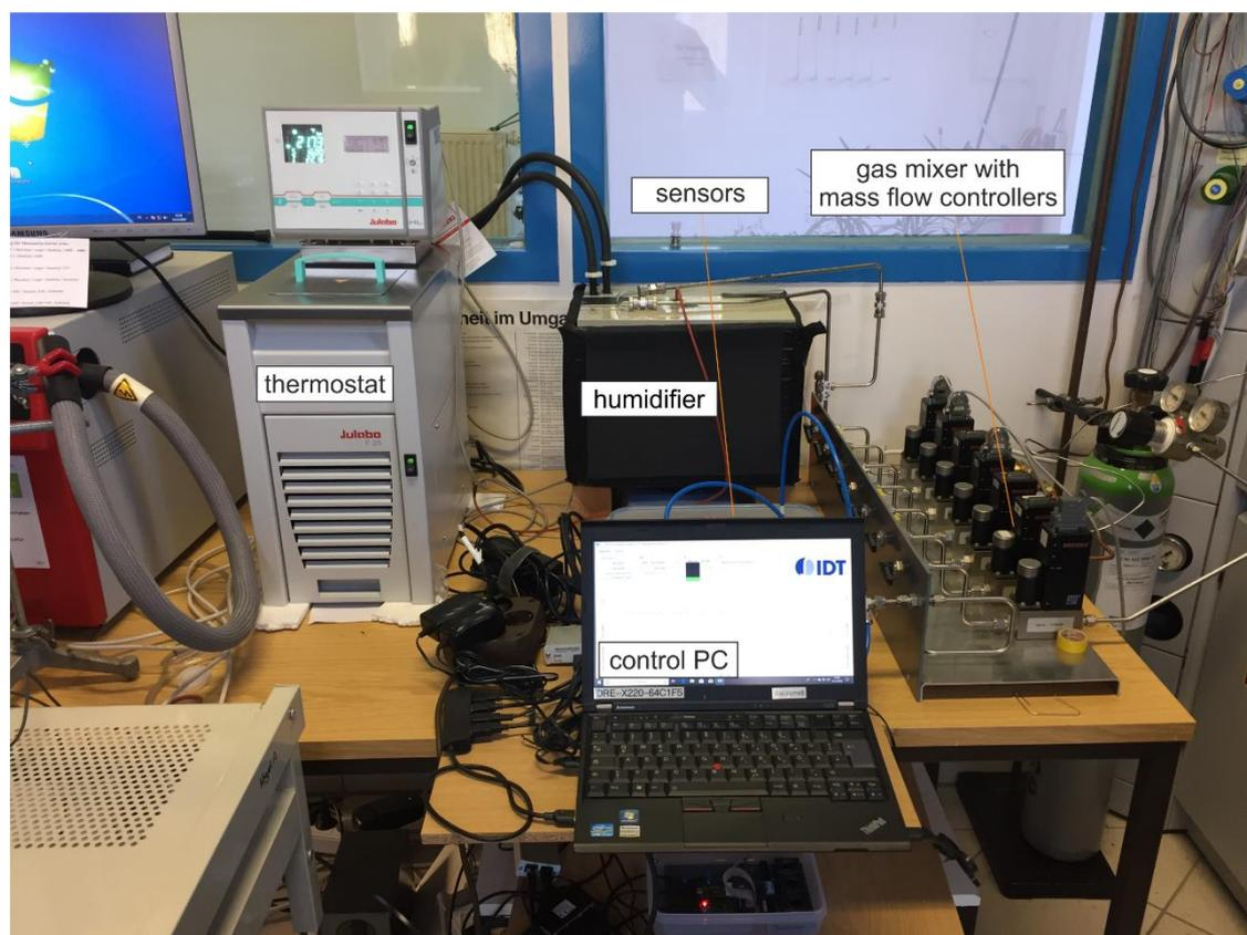
The humidifier for the synthetic air is a purpose-built arrangement of six horizontally positioned glass tubes that is described in detail earlier [3]. The home-built setup for preparation of the ethanol-mixture and its usage is described in detail in [4].
