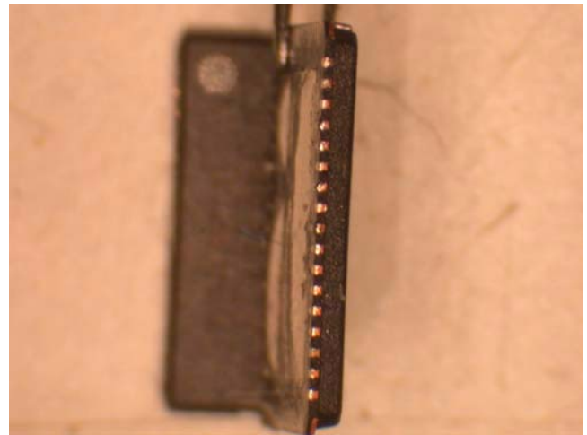
FIGURE 17. FINISHED TINNED THERMAL LAND ON QFN
