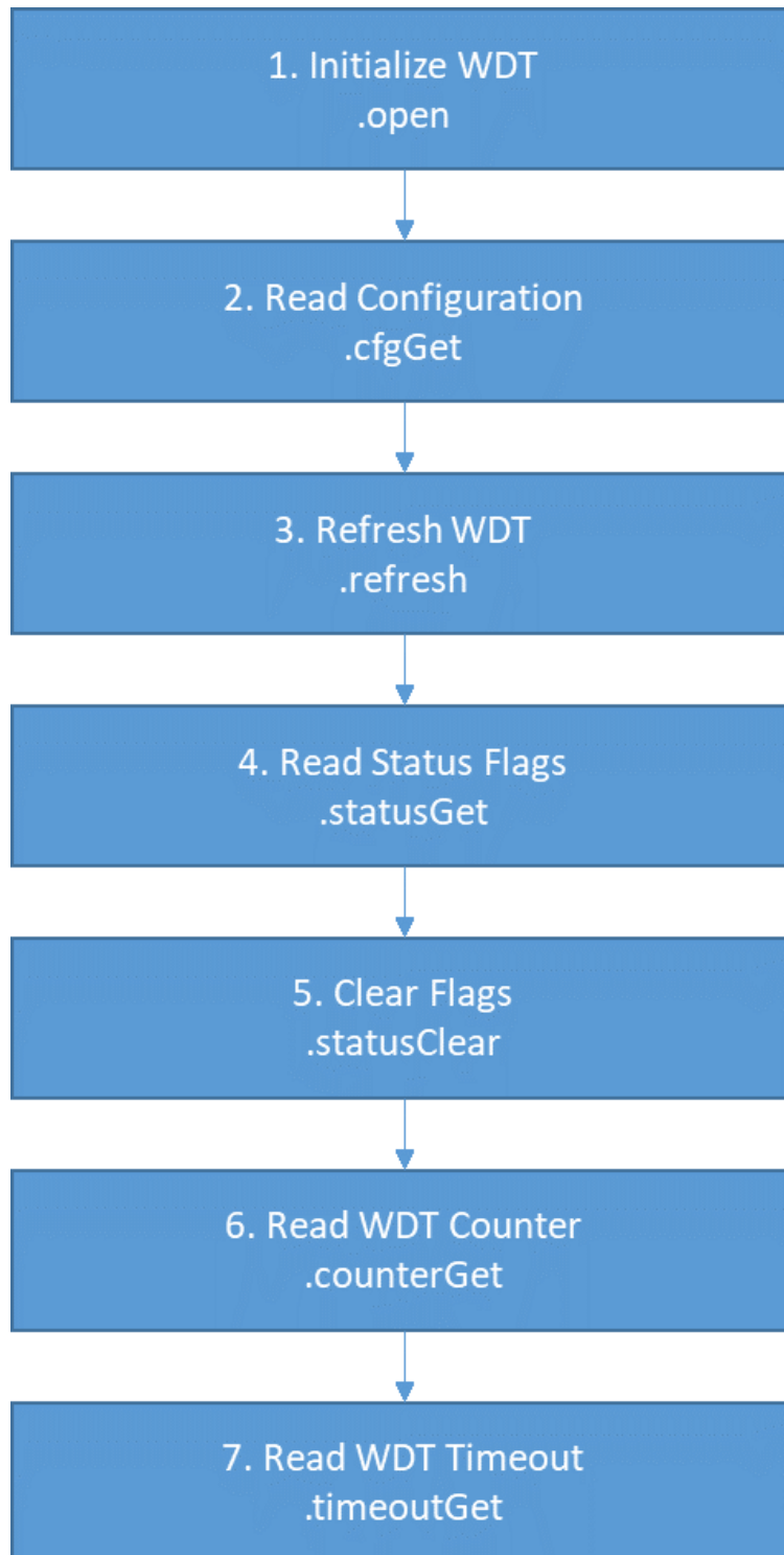
Figure 425: Flow Diagram of a Typical WDT HAL Module Application
