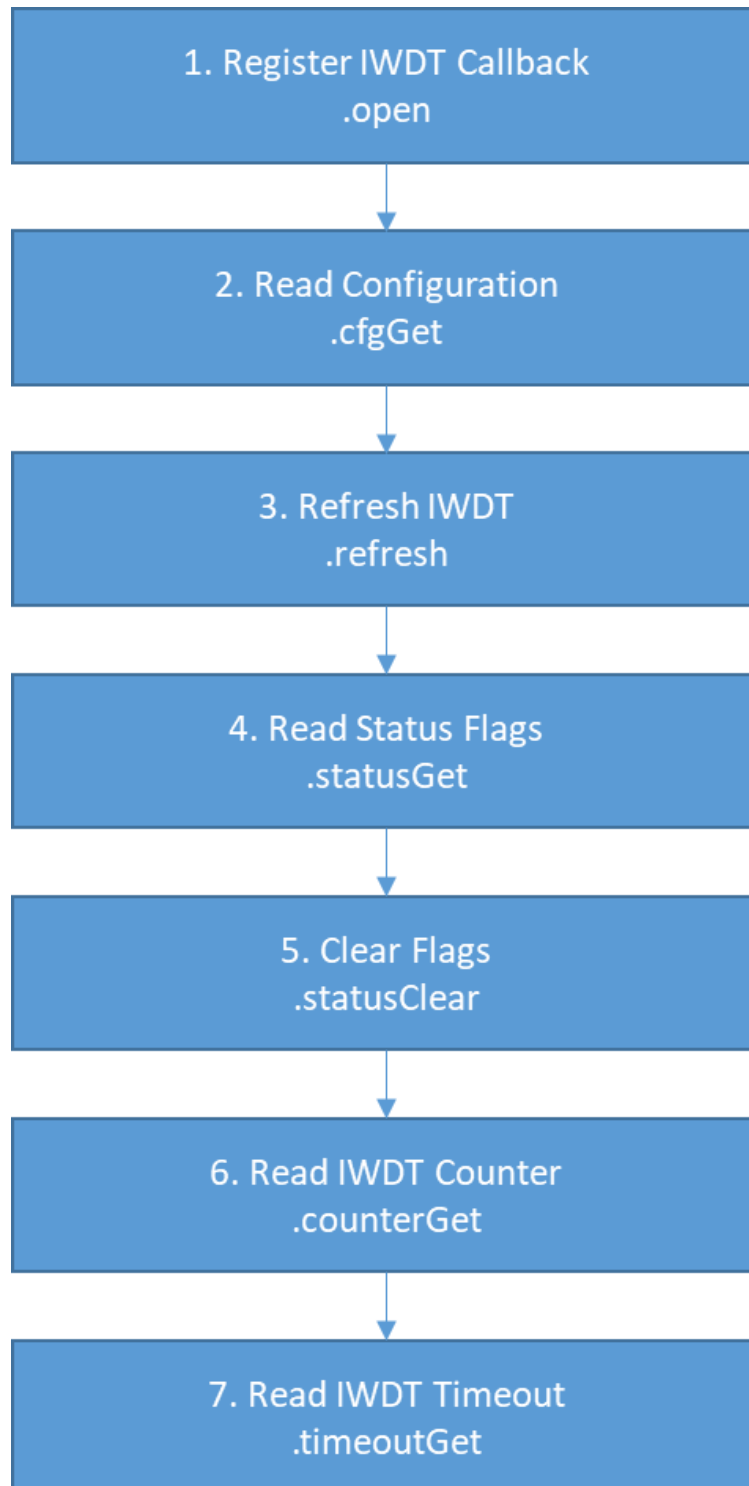
Figure 362: Flow Diagram of a Typical IWDT HAL Module Application
