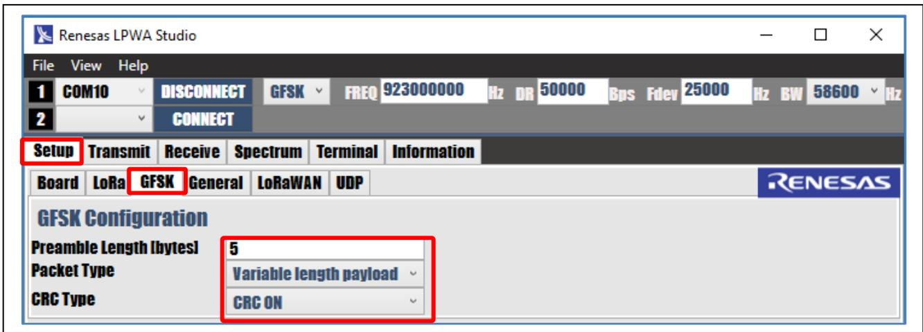
Figure 8. GFSK Packet Parameters Configuration
