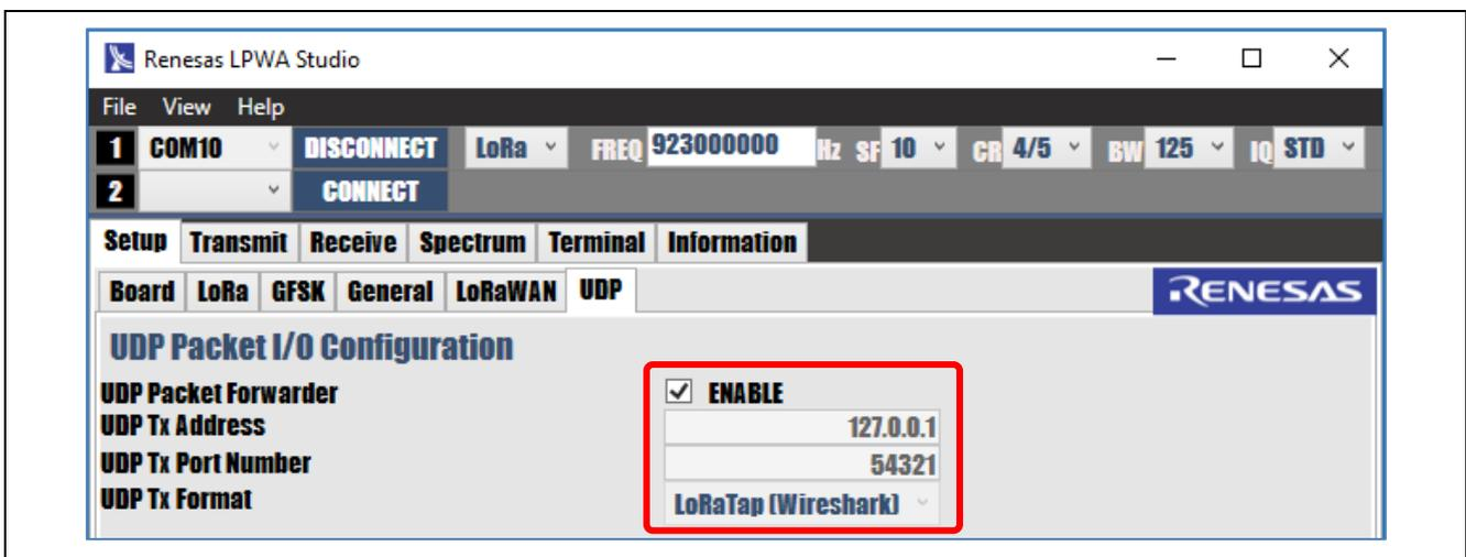
Figure 33. Configuring the UDP Packet Forwarder for Wireshark
