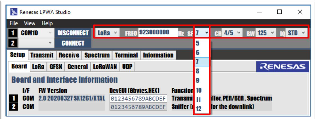
Figure 5. LoRa Parameters
