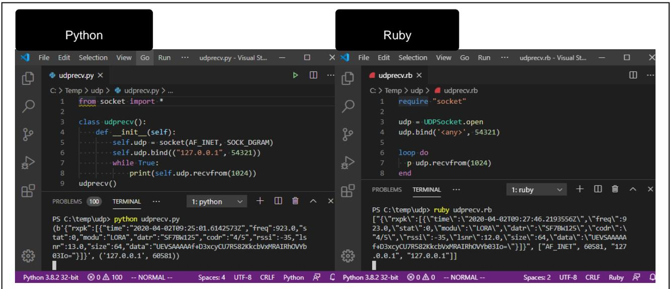
Figure 36. Example Scripts to Receive UDP Packets
