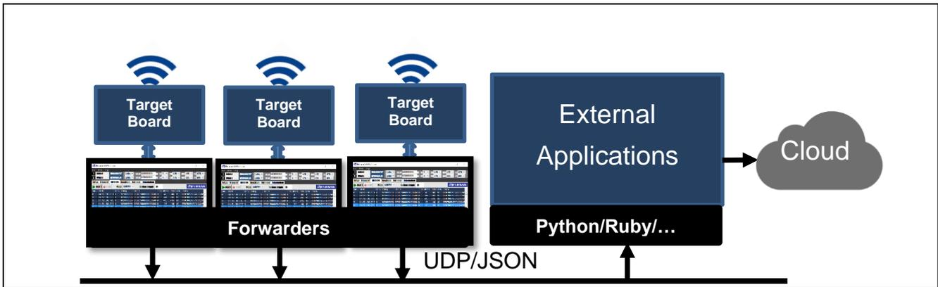
Figure 32. Forwarding the Received LoRaWAN Packets (External Applications)
