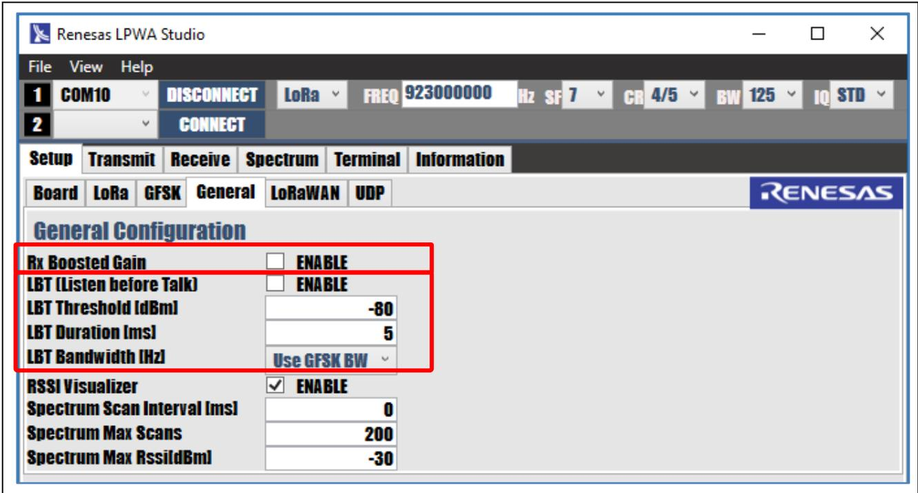
Figure 9. RX Boosted Gain and LBT Parameters Configuration
