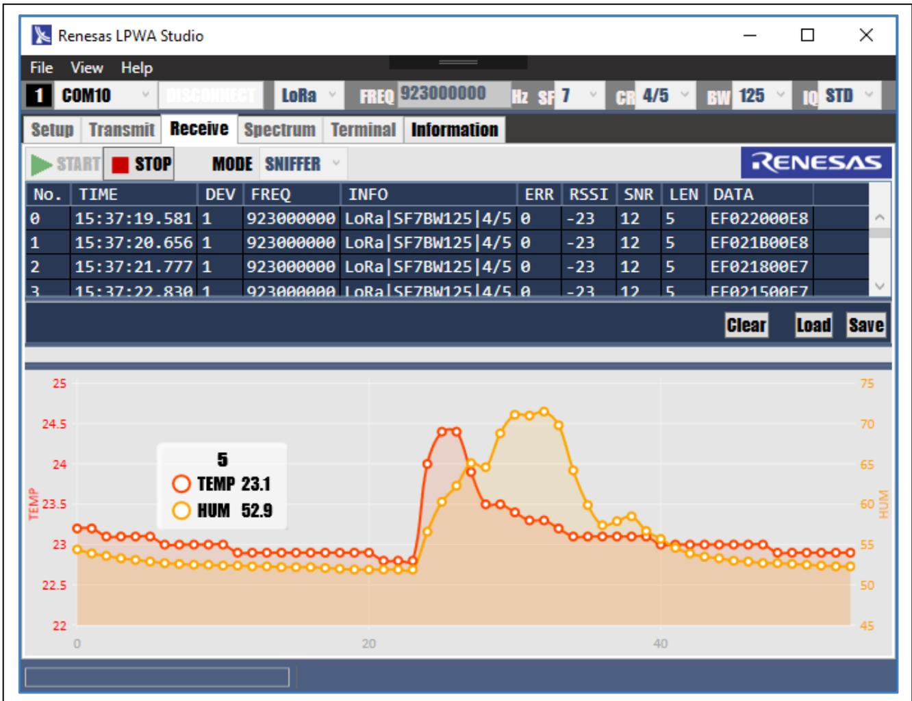
Figure 14. Sensor Data Visualization
