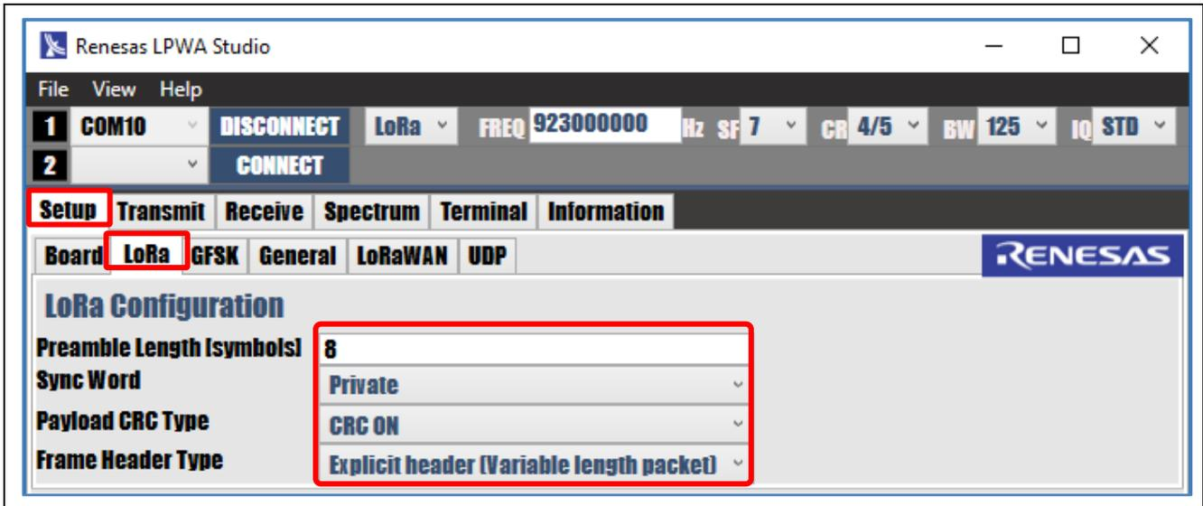
Figure 7. LoRa Packet Parameters Configuration
