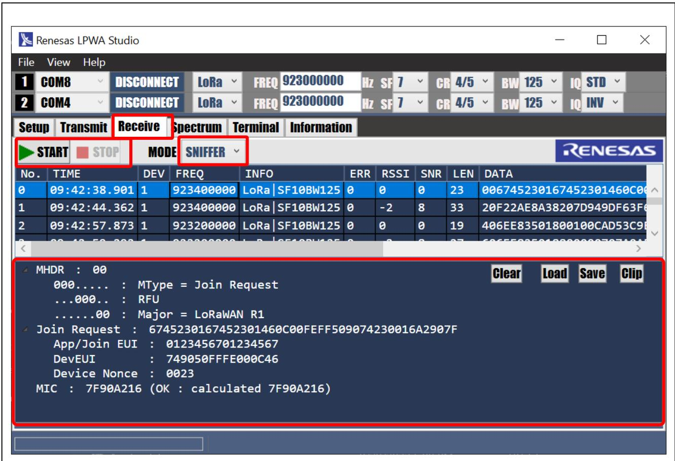
Figure 30. Displaying the Received LoRaWAN Packet
