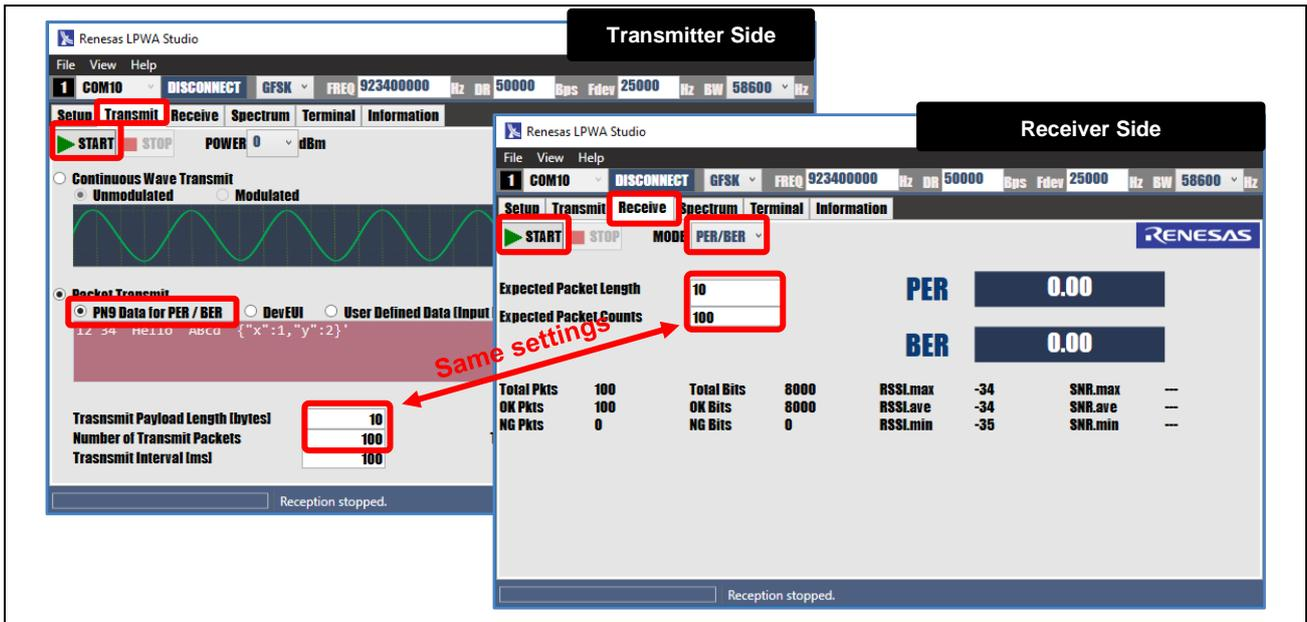
Figure 16. Transmitter and Receiver Side Settings
