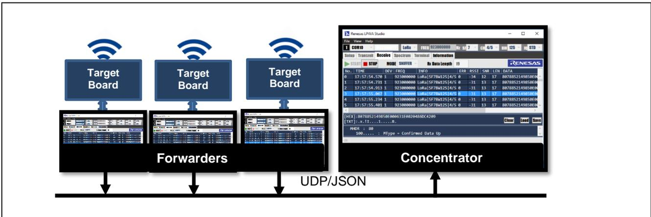
Figure 23. Multiple Target Boards (Multi Channel Capture)
