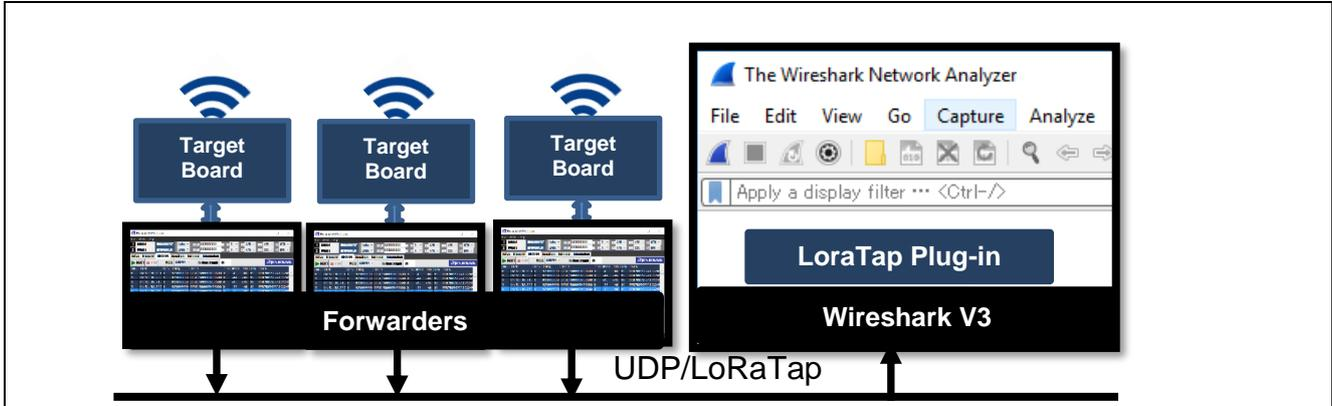
Figure 31. Forwarding the Received LoRaWAN Packets (Wireshark)
