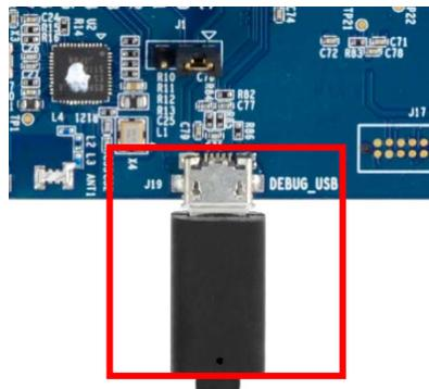
1. Connect the Micro USB end of the supplied USB cable to the PK-S5D9 board J19 connector (DEBUG\_USB).
