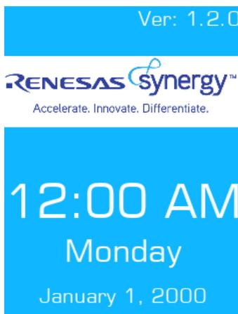
2. Tap the splash screen to enter the Thermostat demo. In this demonstration, the SSP uses the A/D converter to read the internal temperature sensor of the S5D9 and display this information on the LCD Display.
