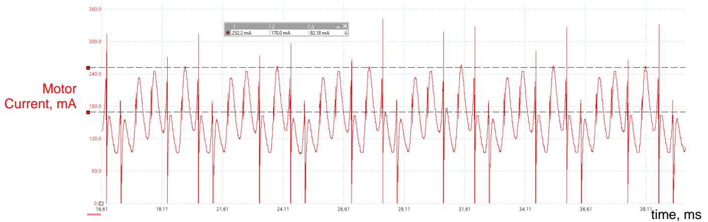
Figure 12: Motor No-Load Current, Power Supply 6.0 V
