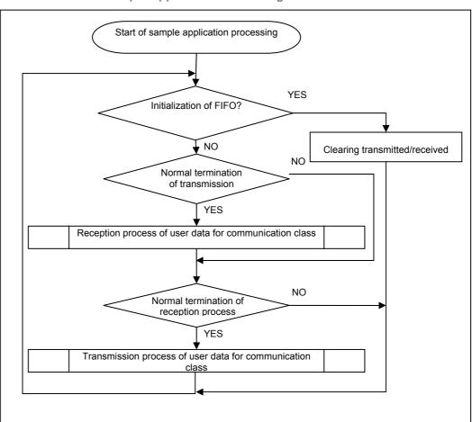
Figure 4-1 Flowchart for the Sample Application Processing
