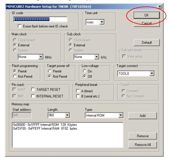
Figure 5-8 IAR C-SPY debug interface configuration (2)
