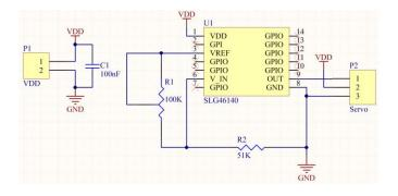
Fig. 2. Servo Control typical application
