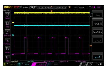
Fig 5. Timing waveforms for servomotor position 90 degrees
