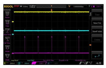
Fig 4. Timing waveforms for servomotor position -90 degrees
