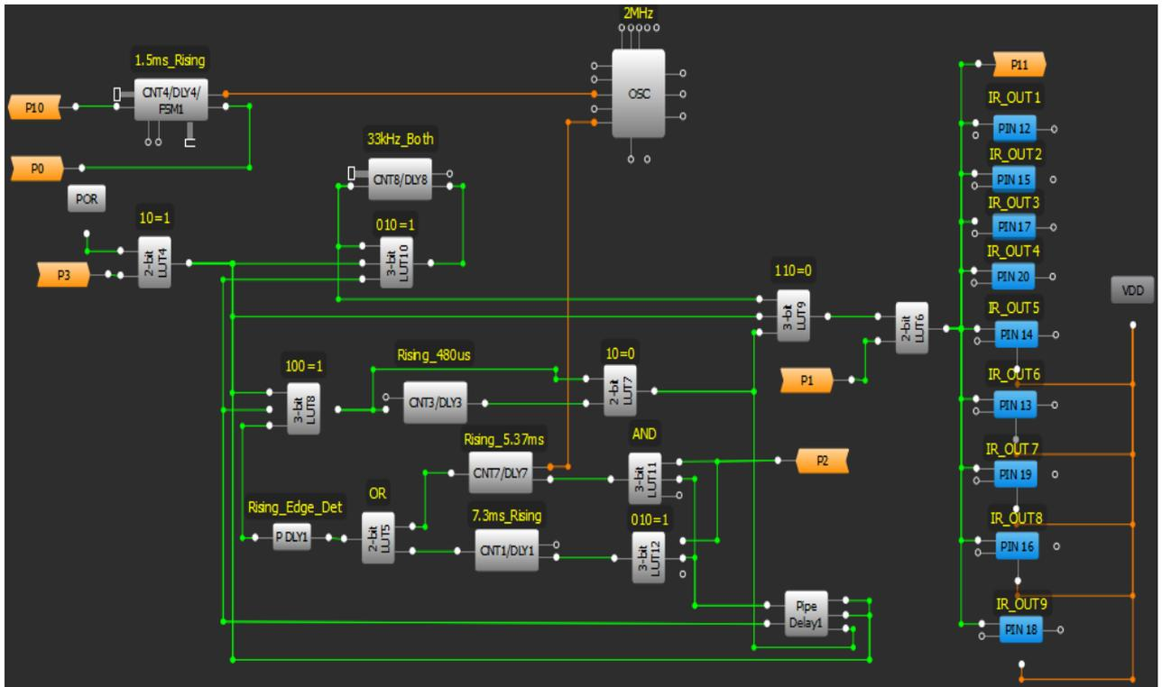
Figure 6. Canon remote schematic
