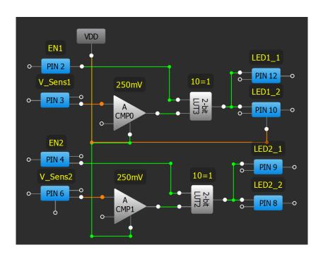
Figure 1. LED constant current circuit design
