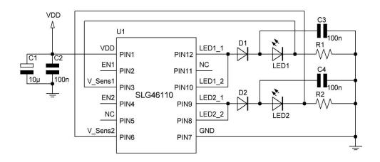
Figure 2. LED constant current typical application circuit
