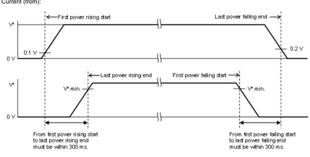
Note: For all V\*, power off state must be 0 V (GND), power rising must be started from 0 V and power falling must be ended to 0 V (excluding DDR-SDRAM power-supply backup state). Periods from 0 V to 0.1 V at power-on and from 0.2 V to 0 V at power-off should be shortened as much as possible.
