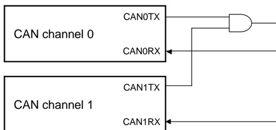
**Figure 48.15 Connection for Inter-Channel Communication Test**
