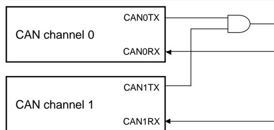
**Figure 48.15 Connection for Inter-Channel Communication Test**
