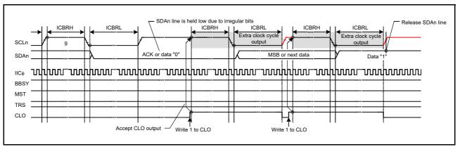
Figure 22.39 Extra SCL Clock Cycle Output Function (CLO Bit)
