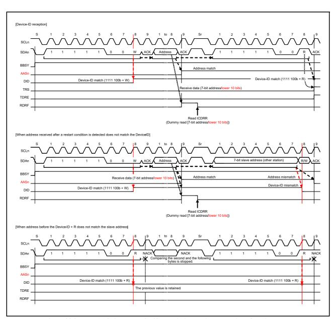
Figure 22.27 AASy/DID Flag Set/Clear Timing during Reception of Device-ID
