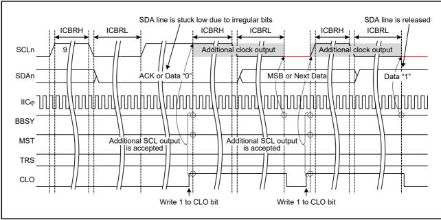
Figure 22.39 Additional SCL Output Function (CLO Bit)
