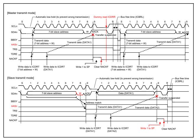
Figure 22.30 Suspension of Data Transfer when NACK is Received (NACKE = 1)
