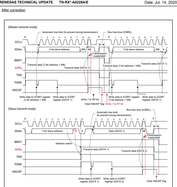
Suspension of Data Transmission When NACK is Received (NACKE = 1) **Figure 22.30**
