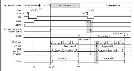
It is correction of "CPU operation status", "Clock request signal (internal signal)" and "INTCSI00" in this Figure.
