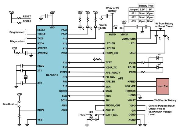
Figure 1. Typical System Diagram
