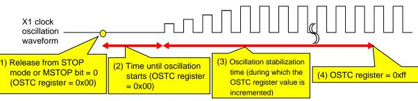
(1) Release from STOP [Simulator (an example of when OSTS is set to 0x07)] X1 clock oscillation waveform Release from STOP mode or MSTOP bit = 0 The OSTC register is set to 0xff at this point.
